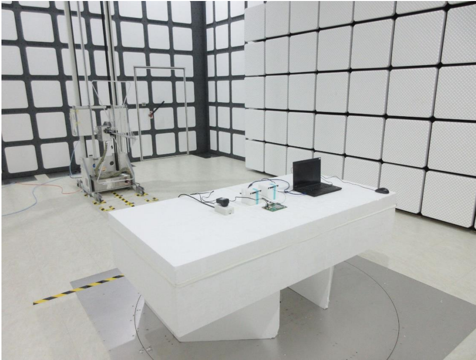
Description: Radiated Emission Test Setup for 1GHz~18GHz
