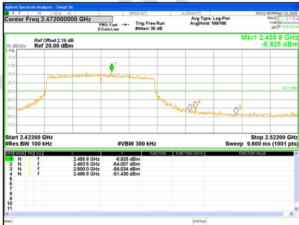
Band Edge NVNT ax40 2452MHz Ant1 Emission
