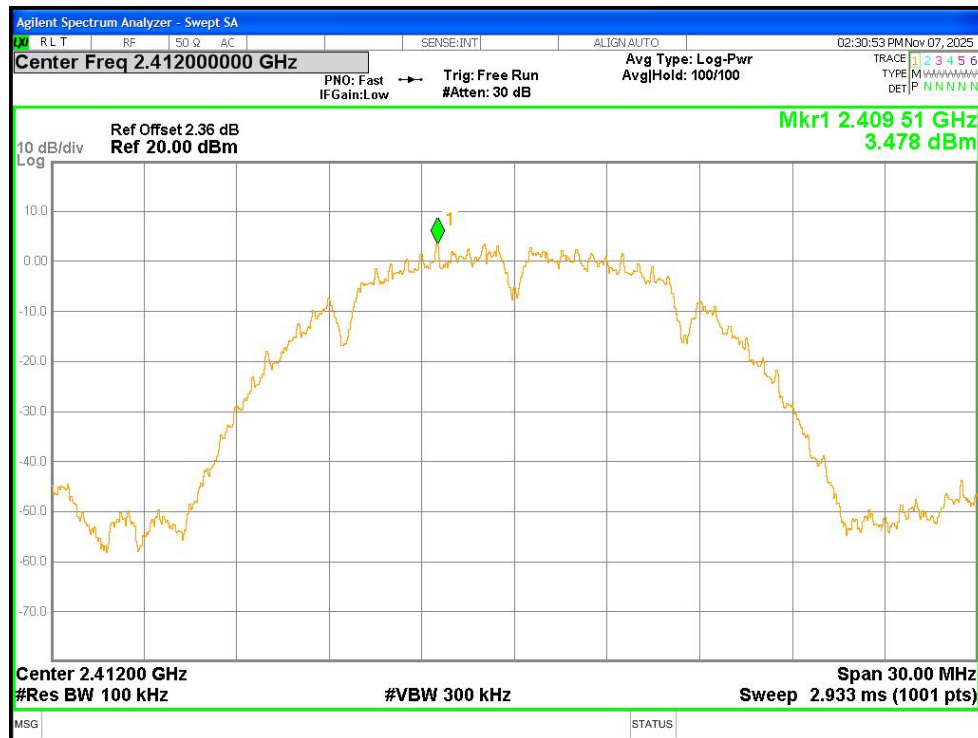
Tx. Spurious NVNT b 2412MHz Ant1 Emission
