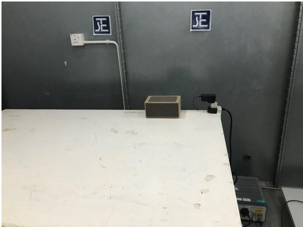
Measurement of Conducted Emission Test Set Up
