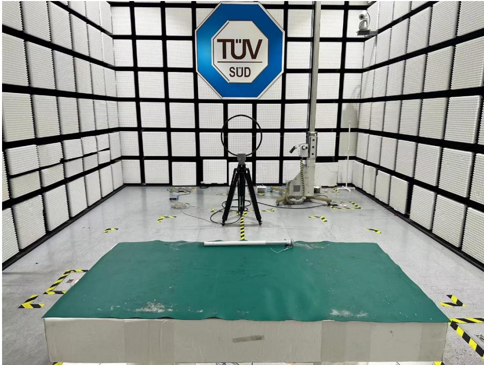
Radiated Emission Setup 9kHz ~ 30MHz
