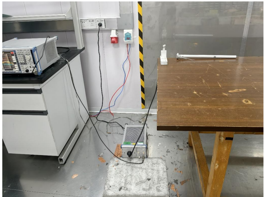
Conducted Emission Test Setup
