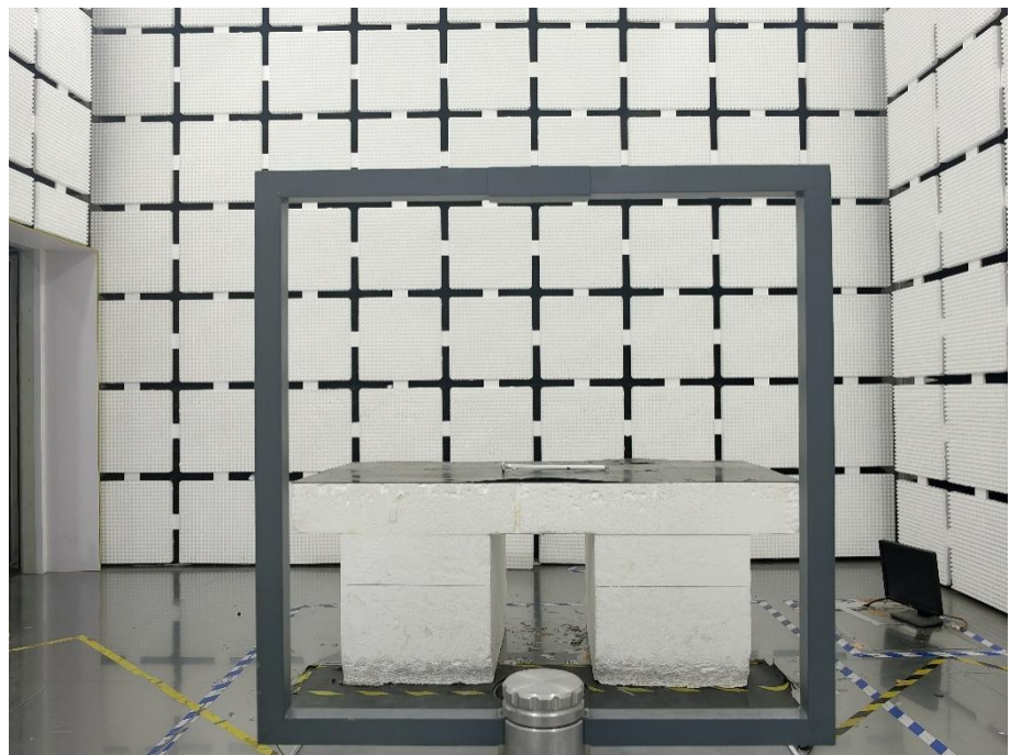
Radiation Emission Test Setup (Below 30MHz)
