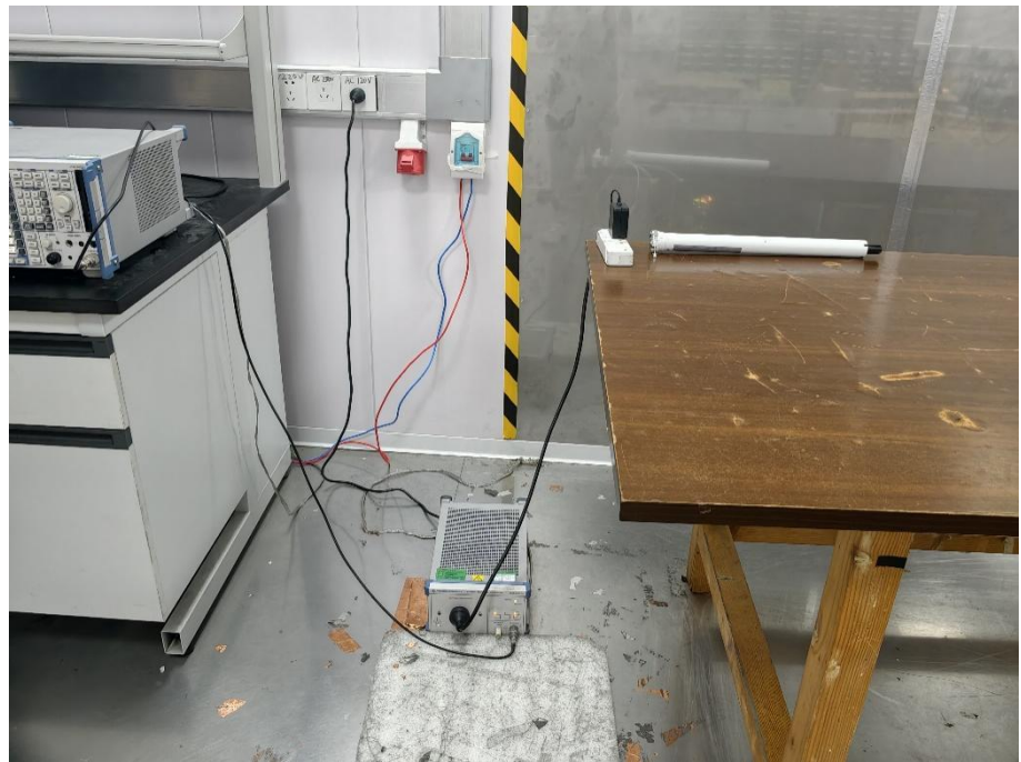
Conducted Emission Test Setup
