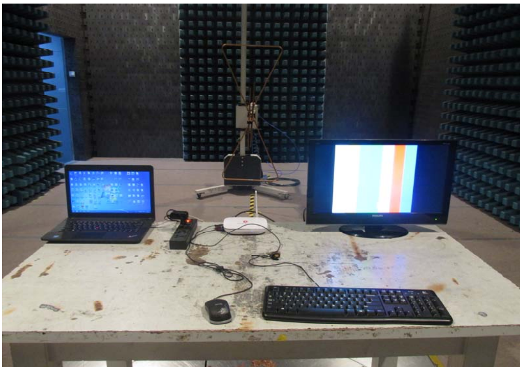
Radiated Emission of 30M-1G
