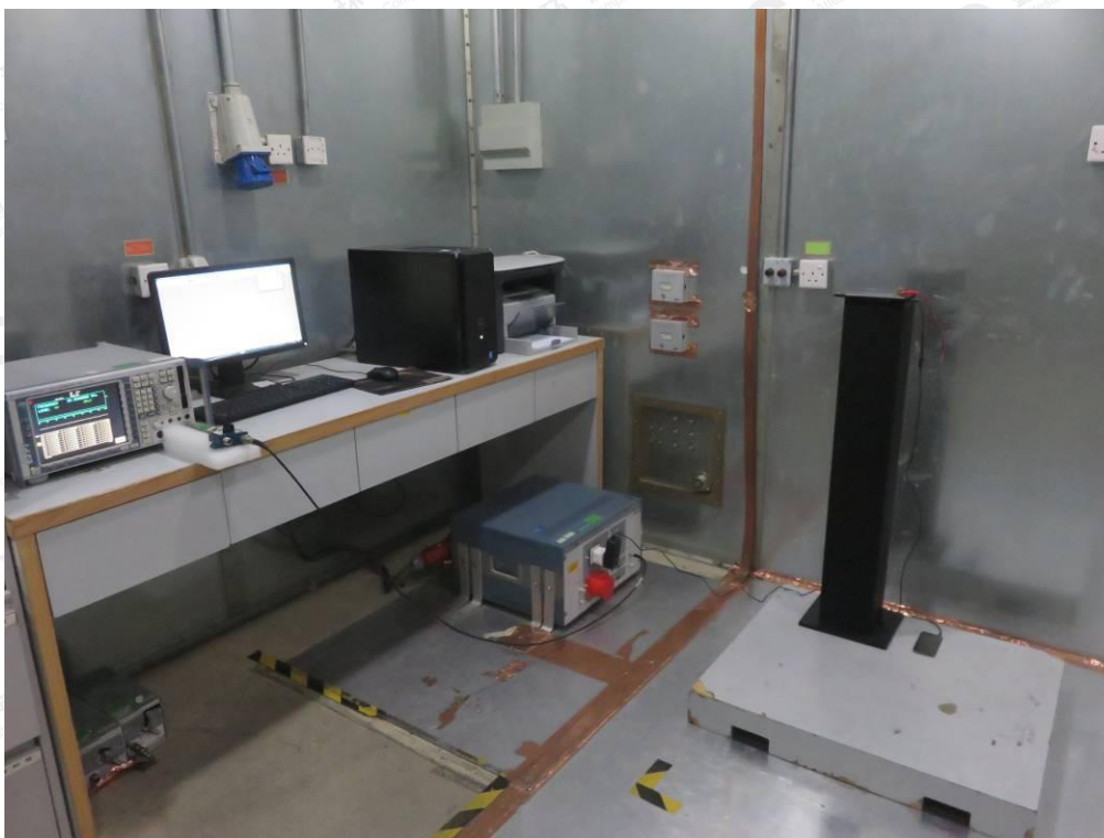
FCC RADIATED EMISSION TEST SETUP
