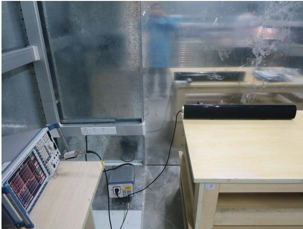
FCC RADIATED EMISSION TEST SETUP
