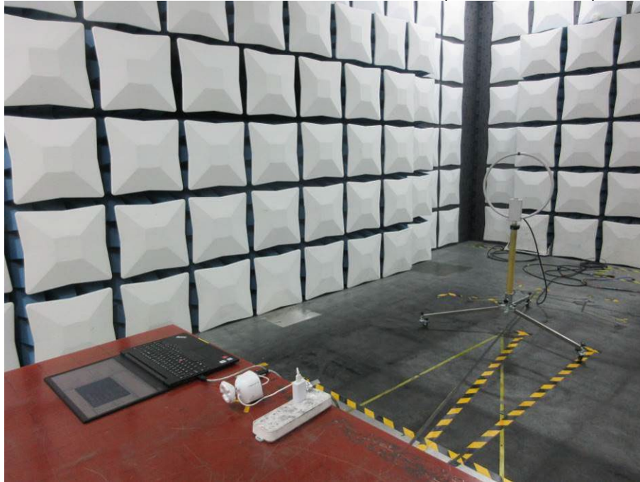
RADIATED RF MEASUREMENT SETUP (9kHz ~ 30 MHz)
