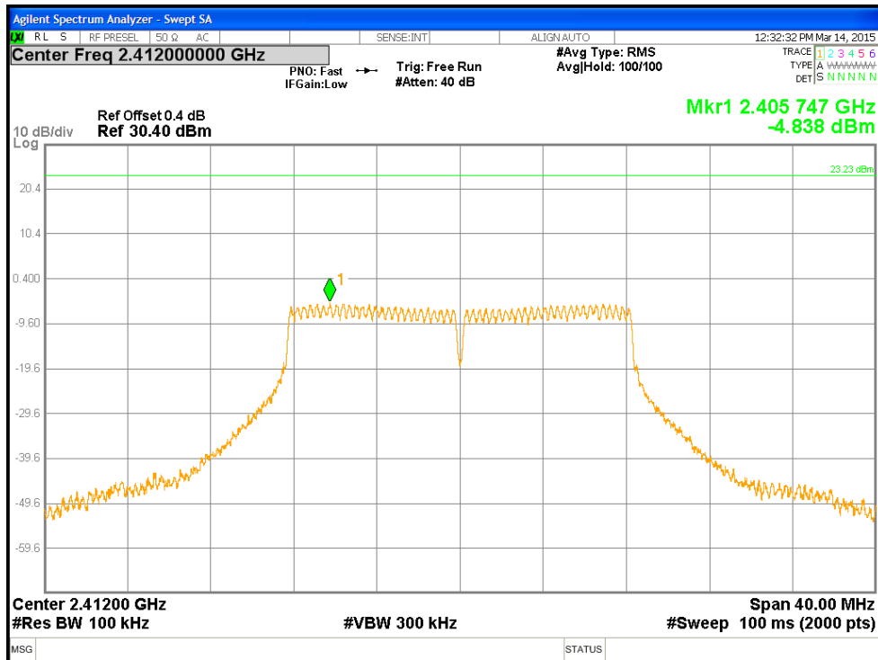
Figure 25: Power Spectral Density, 2412 MHz at 802.11g 6Mbps, Chain 1
