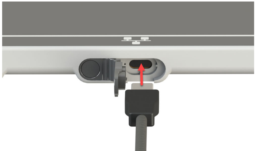
Figure 4 Imaging System Overview – Service Cable Connection
