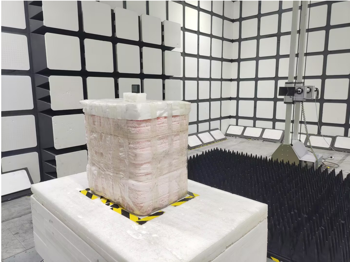
Radiated Emissions View (18-25 GHz)
