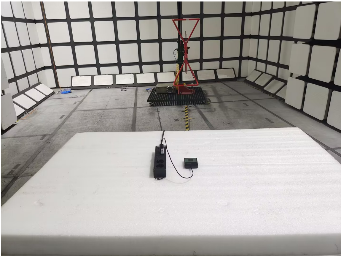
Radiated Emissions View (Below 1 GHz)
