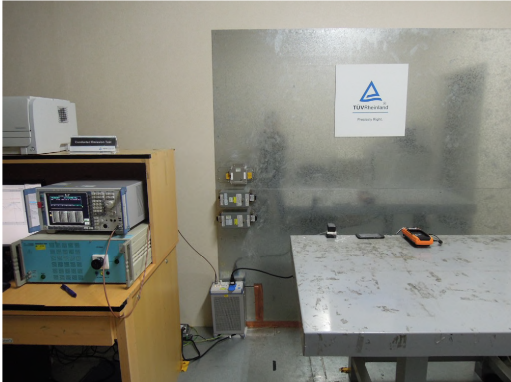
Photograph 6: Set-up for AC Mains (Back View)
