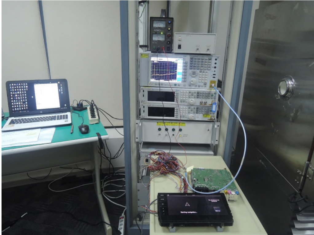
Photograph 8: Set-up for Conducted testing
