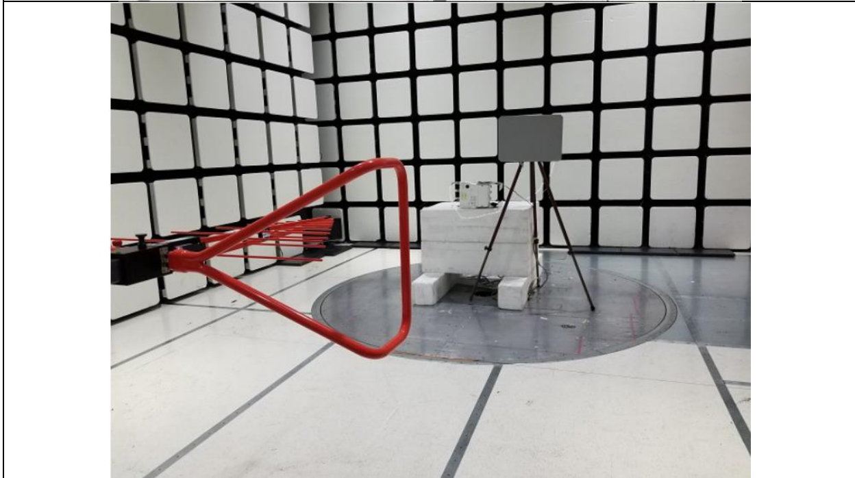
Title: Radiated Spurious Emissions 30MHz-1GHz – Test Setup
