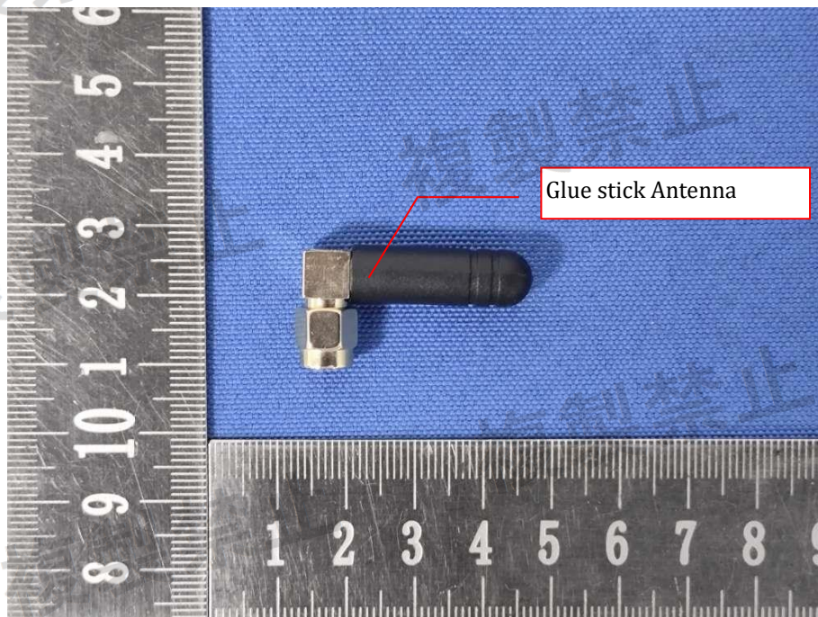
EUT Internal View 17
