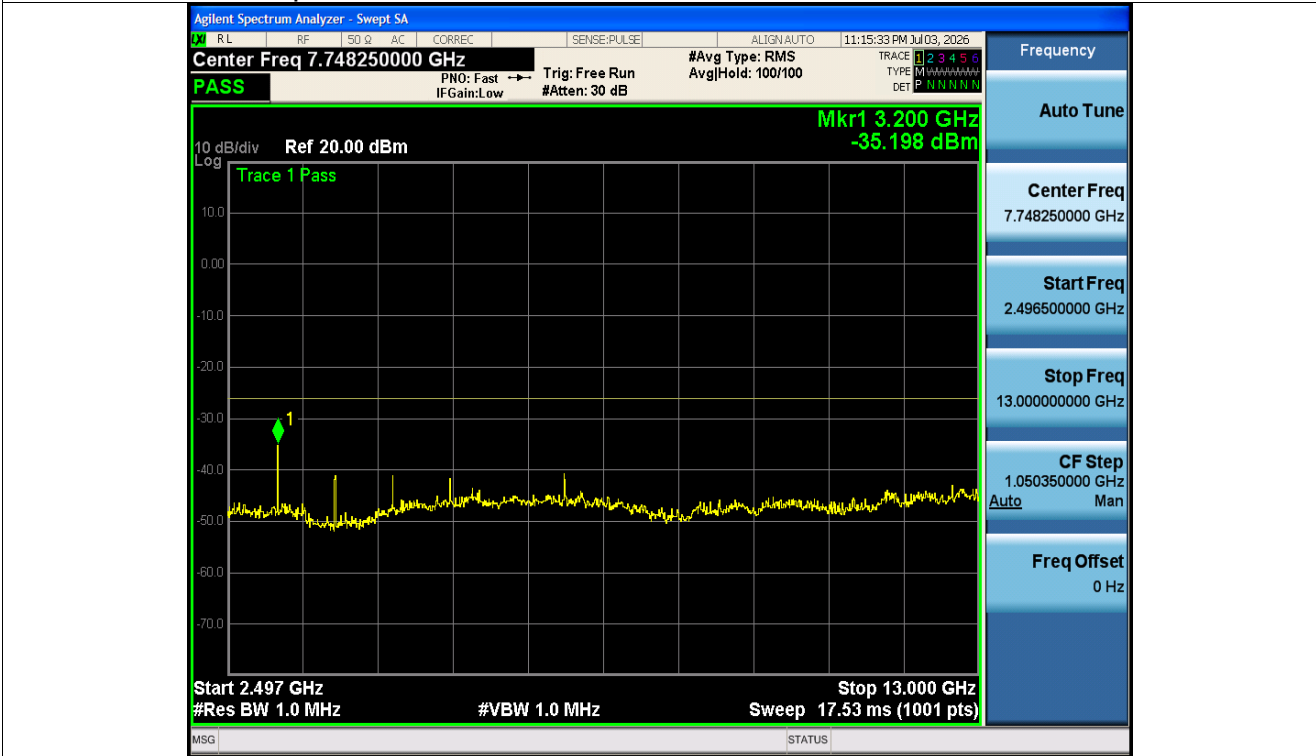
Tx. Spurious NVNT 2402MHz Ant1 @ 2496.5MHz-13000MHz
