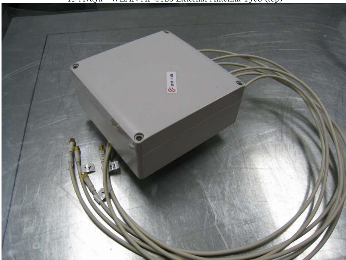
13 Avaya - WLAN AP 8120 External Antenna Tyco (top)
