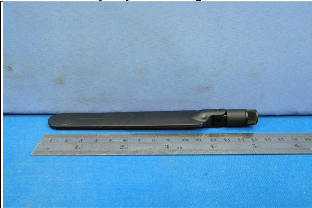
Antenna Set 4 Brand: Long Cheng / Model No.: FDE_ACBSMA-BGP
