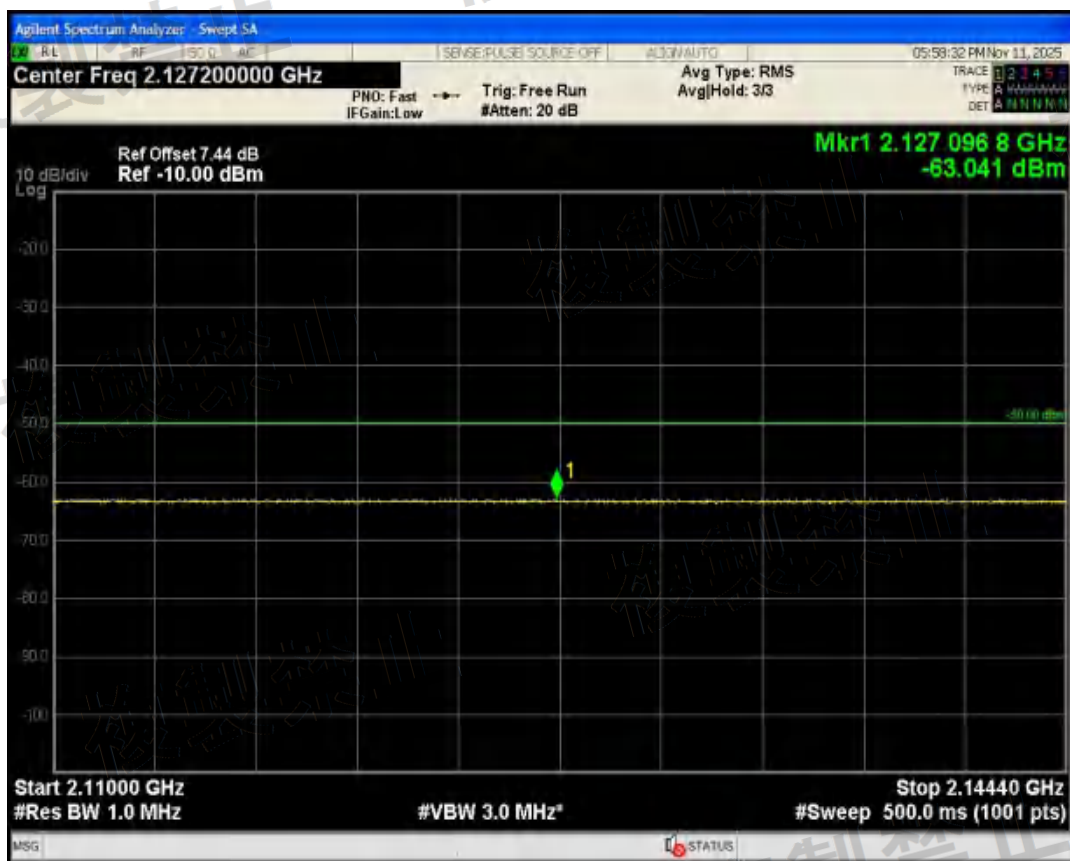
Band1(10L) QPSK BW=10MHz Channel=18073 RB Size=50 Position=#0 Range=2010 MHz-2025 MHz
