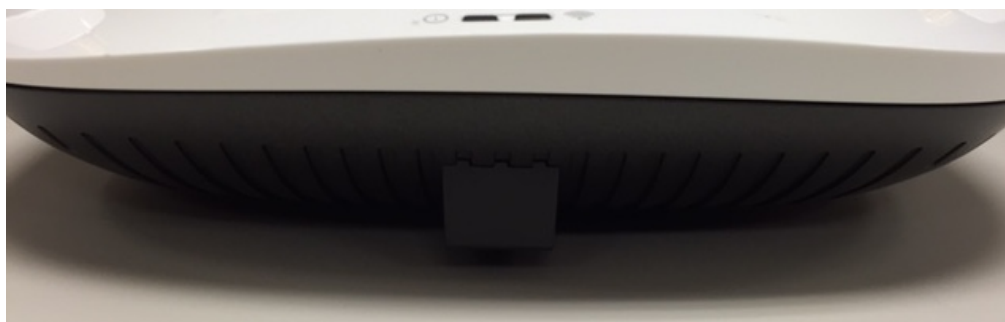
Front View APIN0325 (Showing BLE Antenna)
