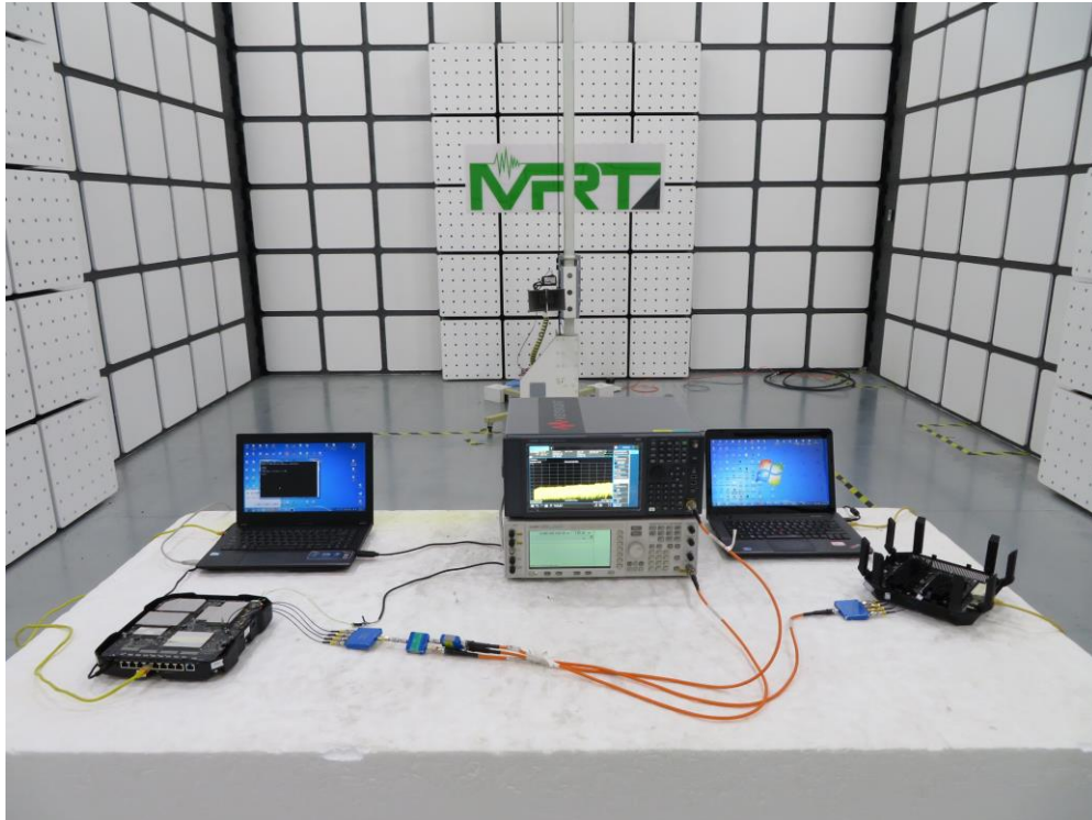
Description: DFS Test Setup
