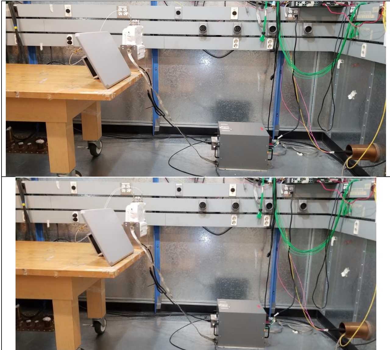
Title: Conducted Emissions 150KHz-30MHz – Test Setup
