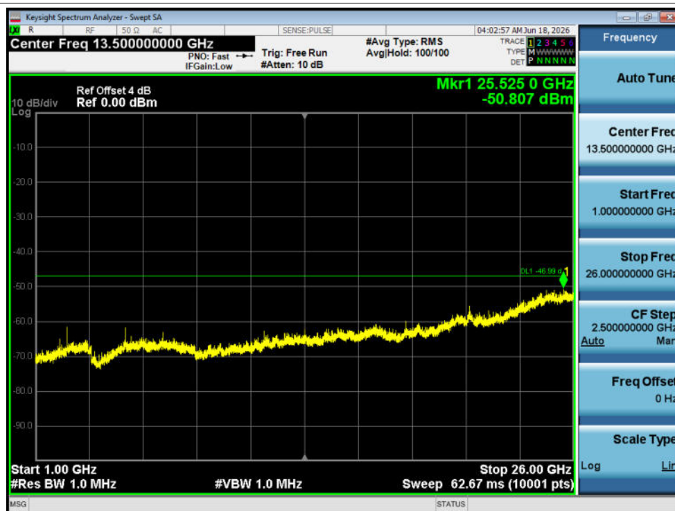
Rx. Spurious NVNT n20 5200MHz Ant1 @ 1000MHz-26000MHz
