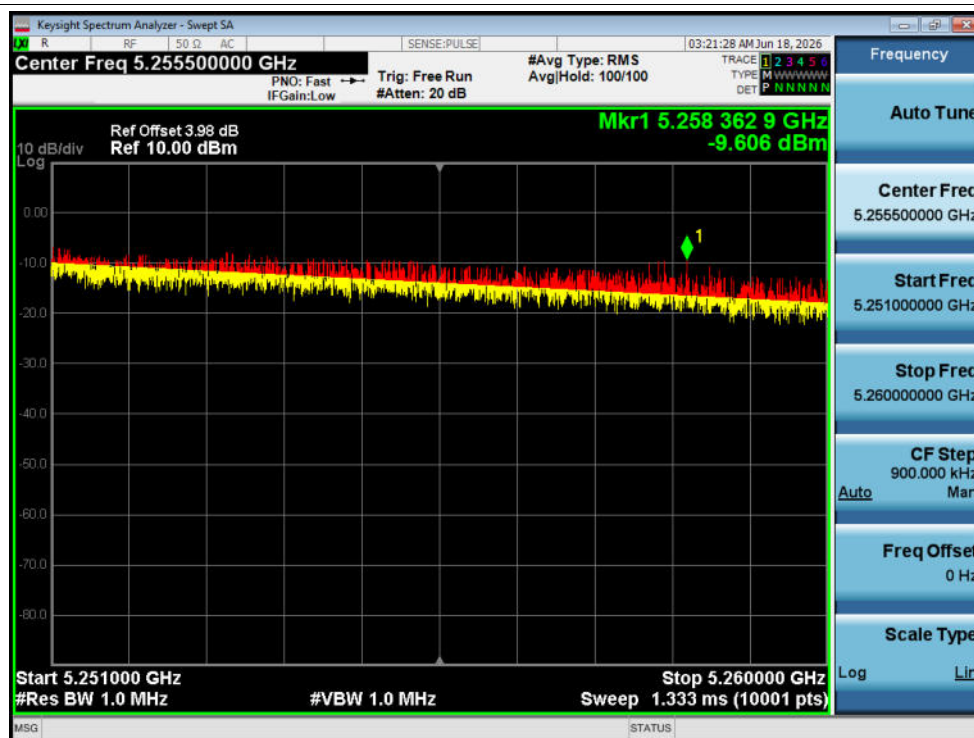
Tx. Spurious NVNT a 5240MHz Ant1 @ 5251MHz-5260MHz
