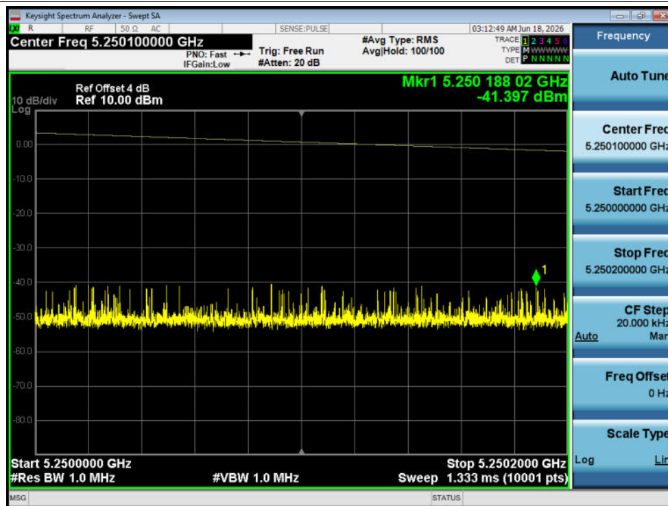
Tx. Spurious NVNT a 5200MHz Ant1 @ 5250MHz-5250.2MHz
