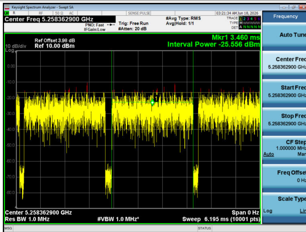
Tx. Spurious NVNT a 5240MHz Ant1 @ 5251MHz-5260MHz Final
