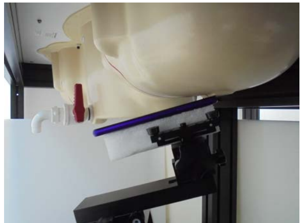
Figure 4. Left Head SAR Test Setup (Tilted)
