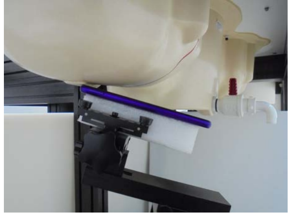
Figure 2. Right Head SAR Test Setup (Tilted)
