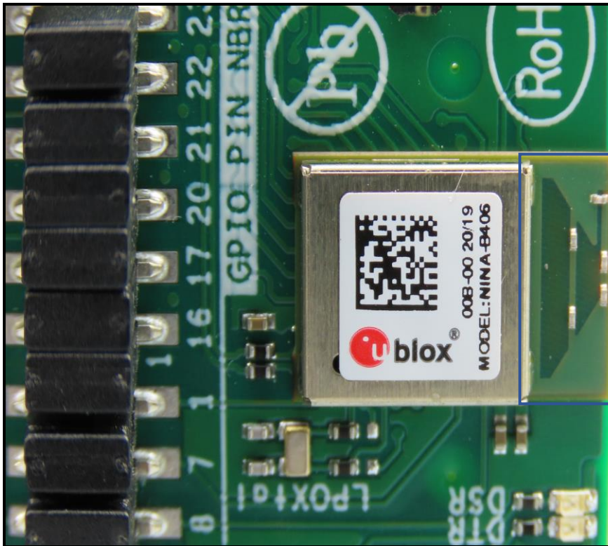
2.4GHz Antenna (Brand: ProAnt, Model: u-blox PCB trace antenna)
