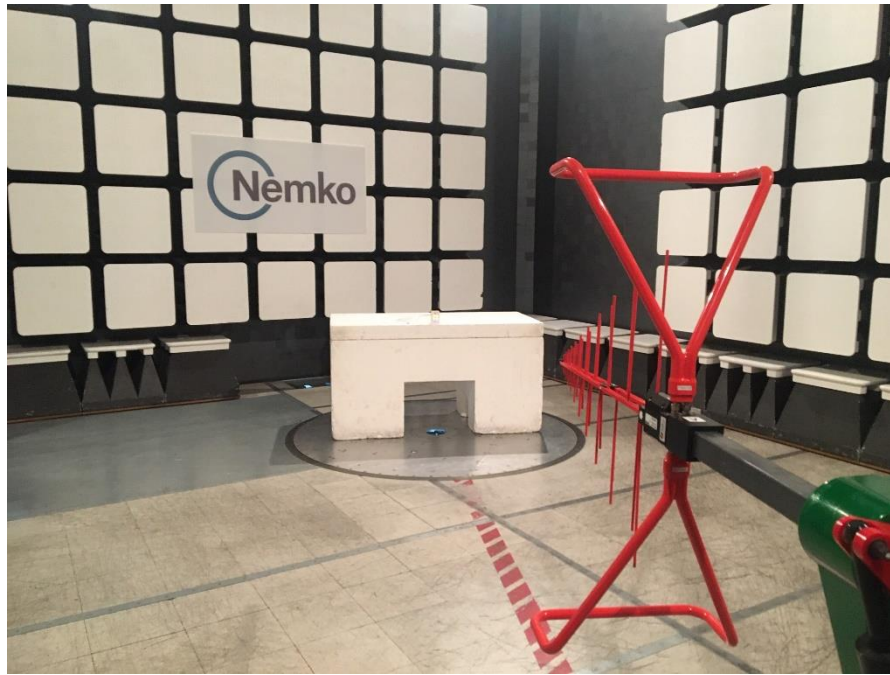
Figure 9.3-1: Radiated spurious emissions setup photo below 1 GHz
