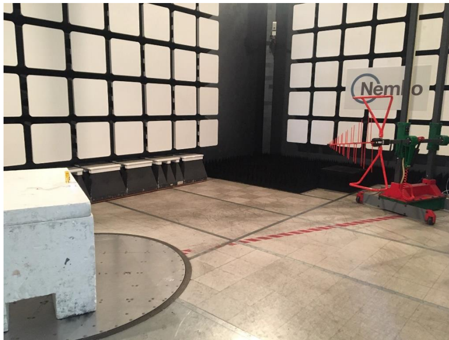
Figure 9.3-2: Radiated spurious emissions setup photo below 1 GHz
