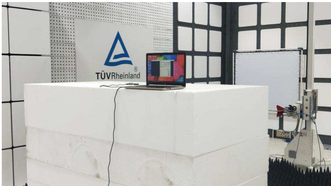
Photograph 4: Set-up for Spurious Emissions (Back View 2)
