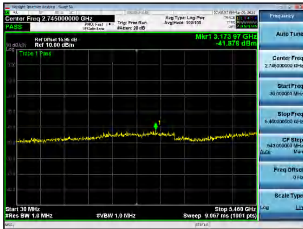
Tx. Spurious NVNT n40 5670MHz Ant1 @ 5460MHz-5470MHz
