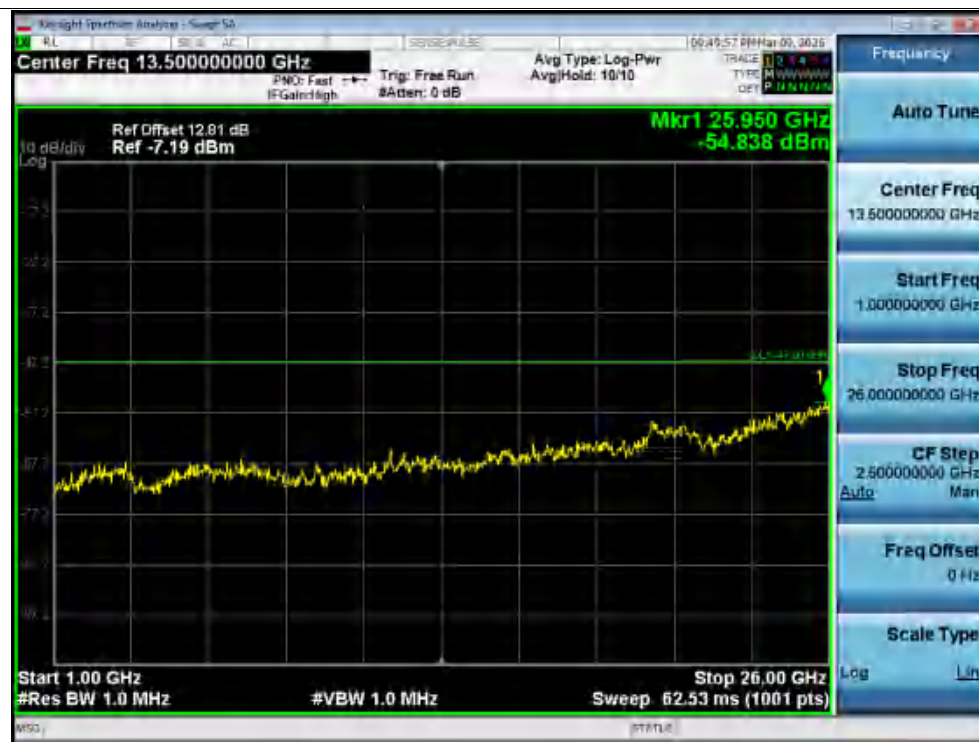
Rx. Spurious NVNT ac80 5610MHz Ant1 @ 1000MHz-26000MHz
