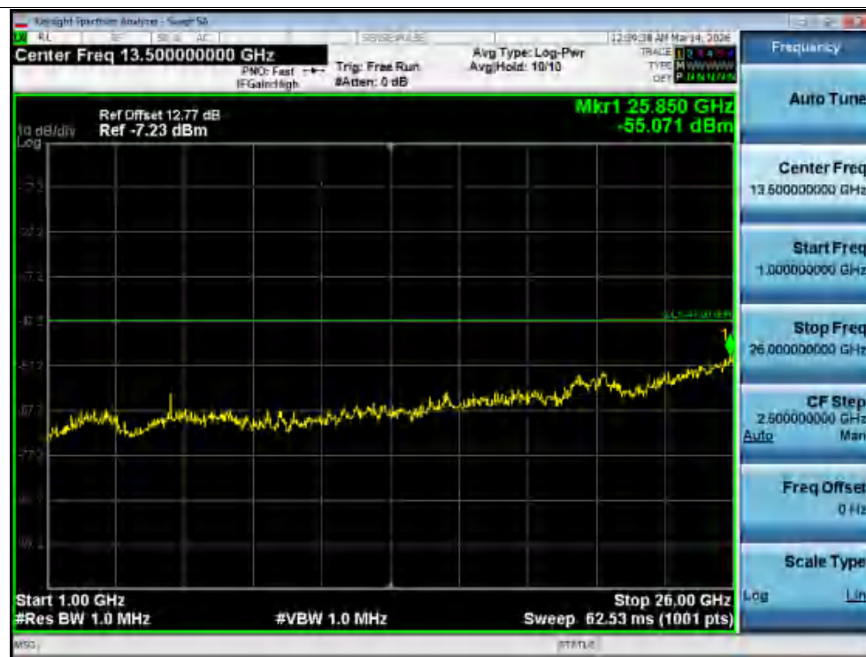
Rx. Spurious NVNT a 5580MHz Ant1 @ 1000MHz-26000MHz
