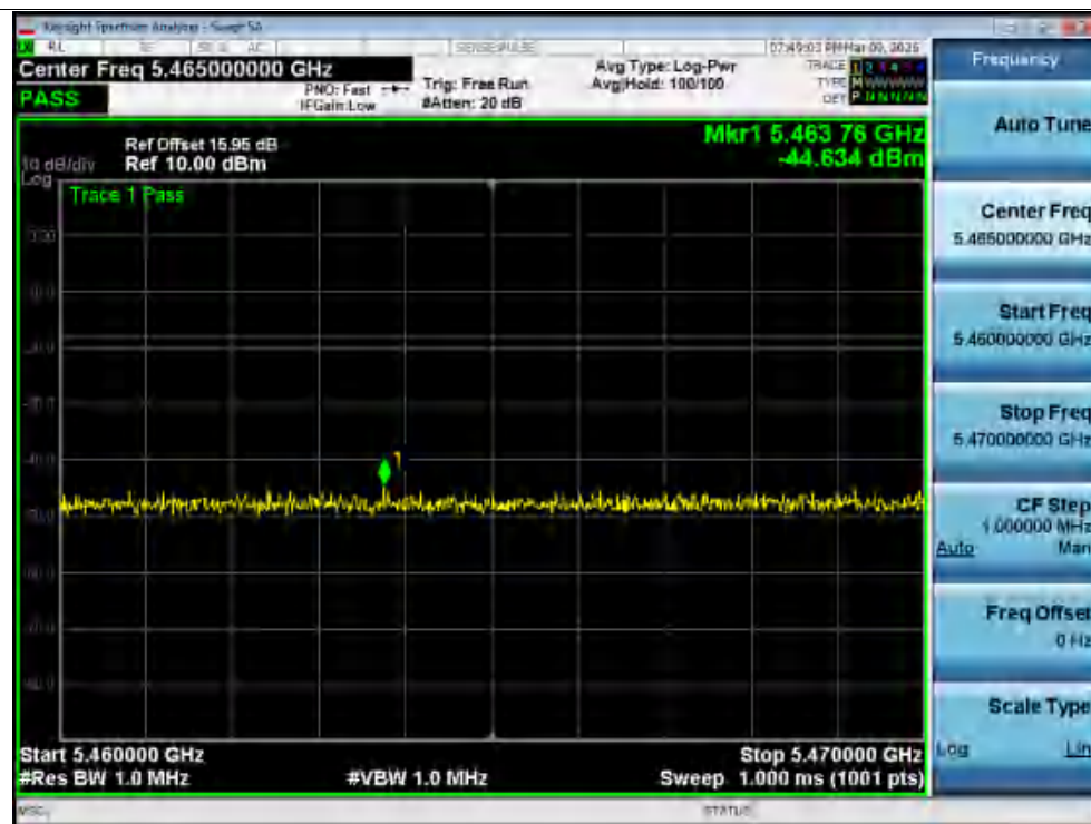
Tx. Spurious NVNT n40 5670MHz Ant1 @ 5460MHz-5470MHz
