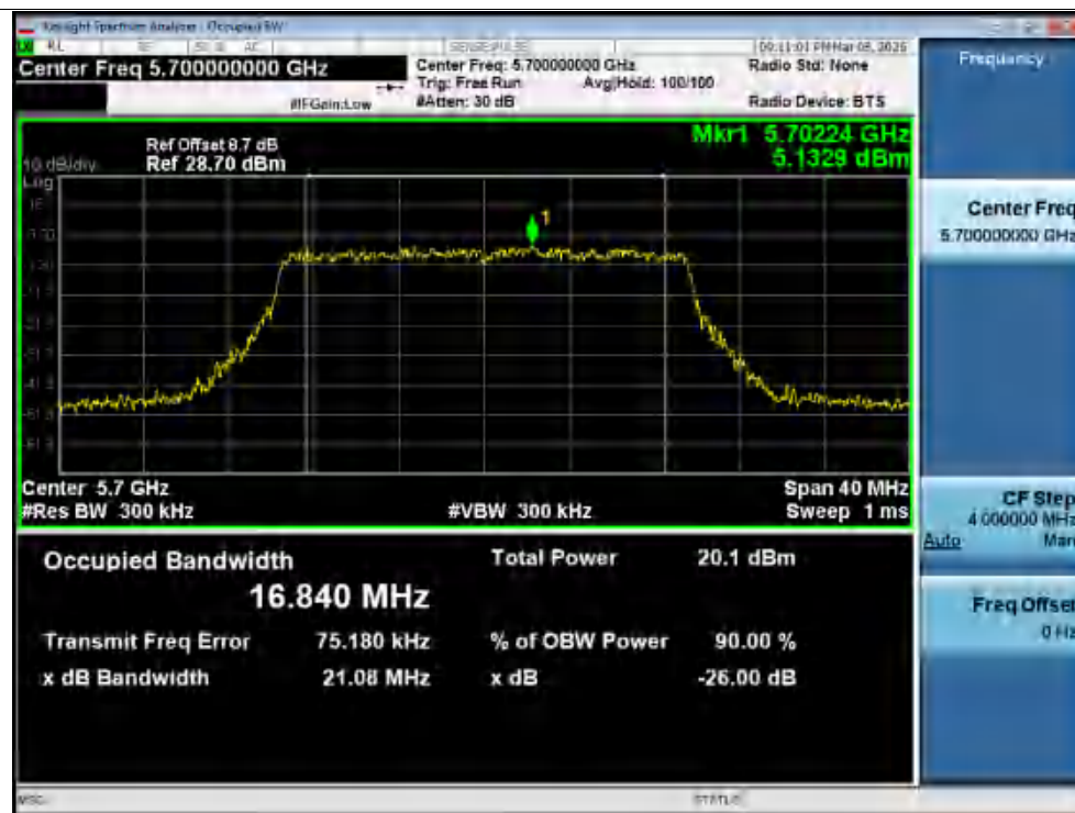
Spreading Bandwidth NVNT ax20 5700MHz Ant2
