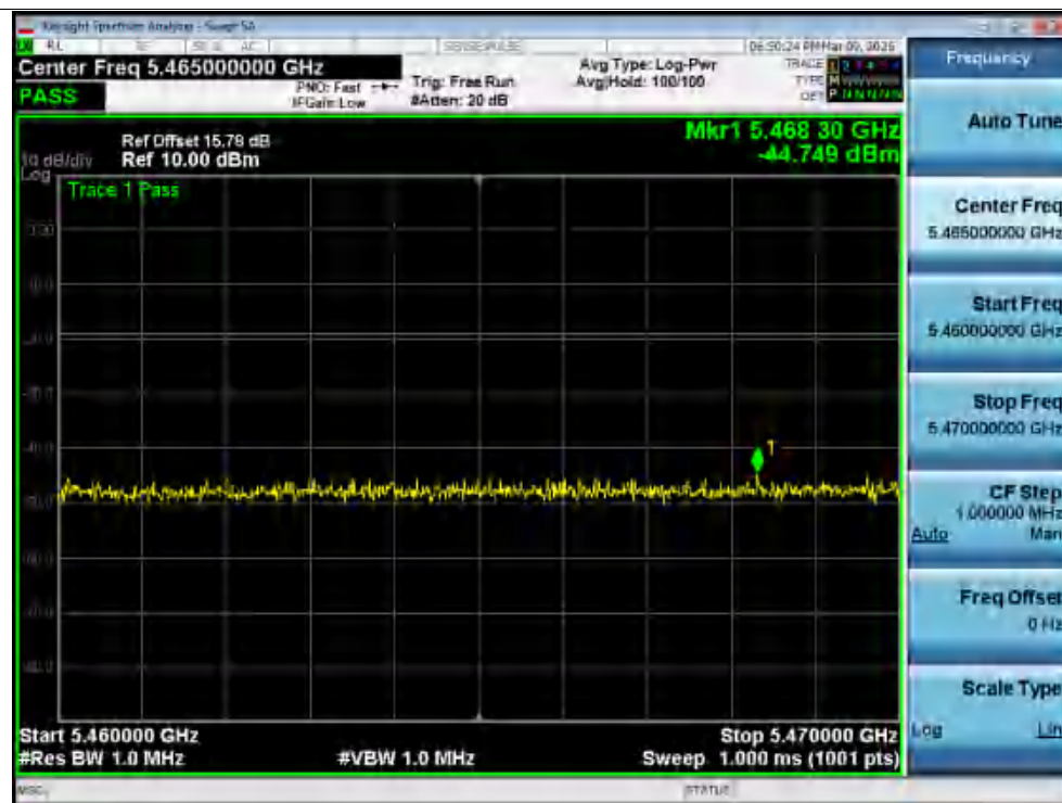
Tx. Spurious NVNT n20 5580MHz Ant1 @ 5460MHz-5470MHz
