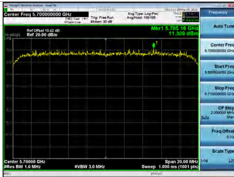
Power NVNT ax20 5700 MHz Ant1 Zero Span
