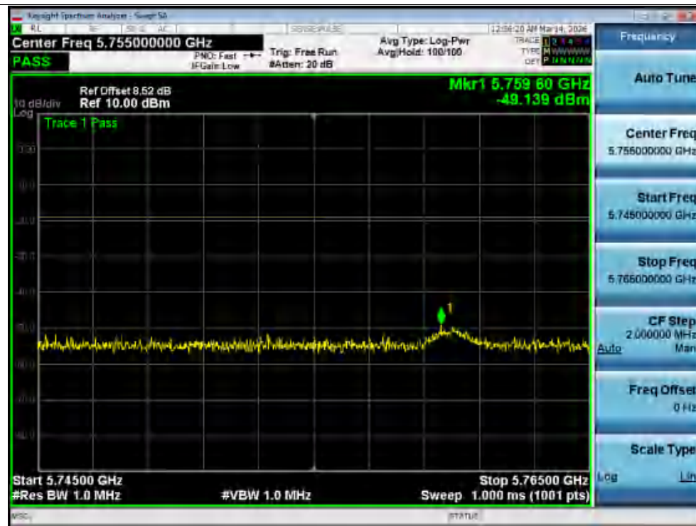
Tx. Spurious NVNT a 5500MHz Ant2 @ 5765MHz-26000MHz
