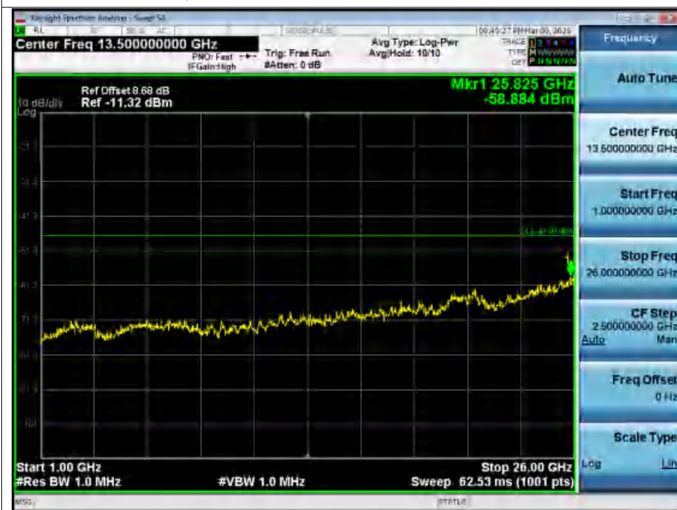
Rx. Spurious NVNT ax40 5670MHz Ant2 @ 1000MHz-26000MHz
