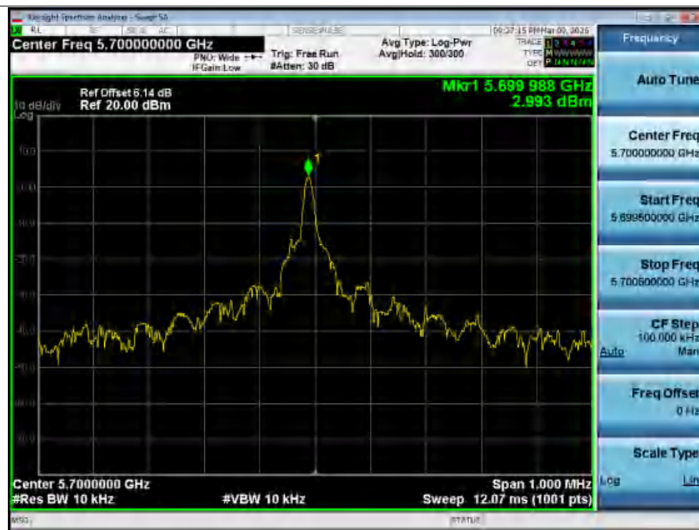
Freq. Error NVNT 5700MHz Ant2
