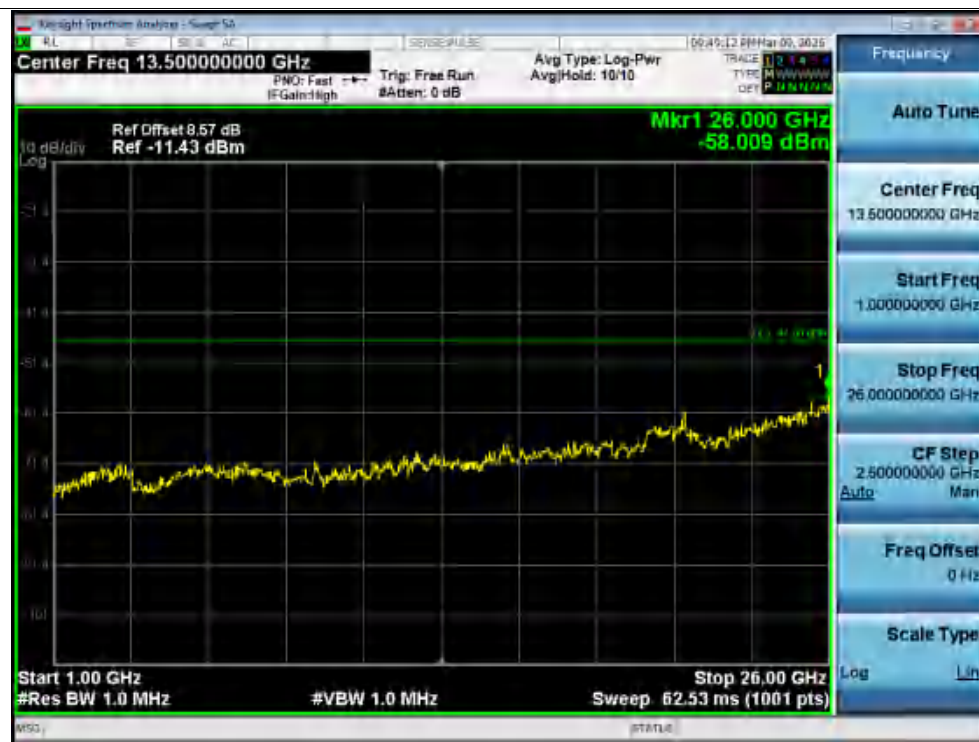
Rx. Spurious NVNT ax40 5590MHz Ant2 @ 1000MHz-26000MHz
