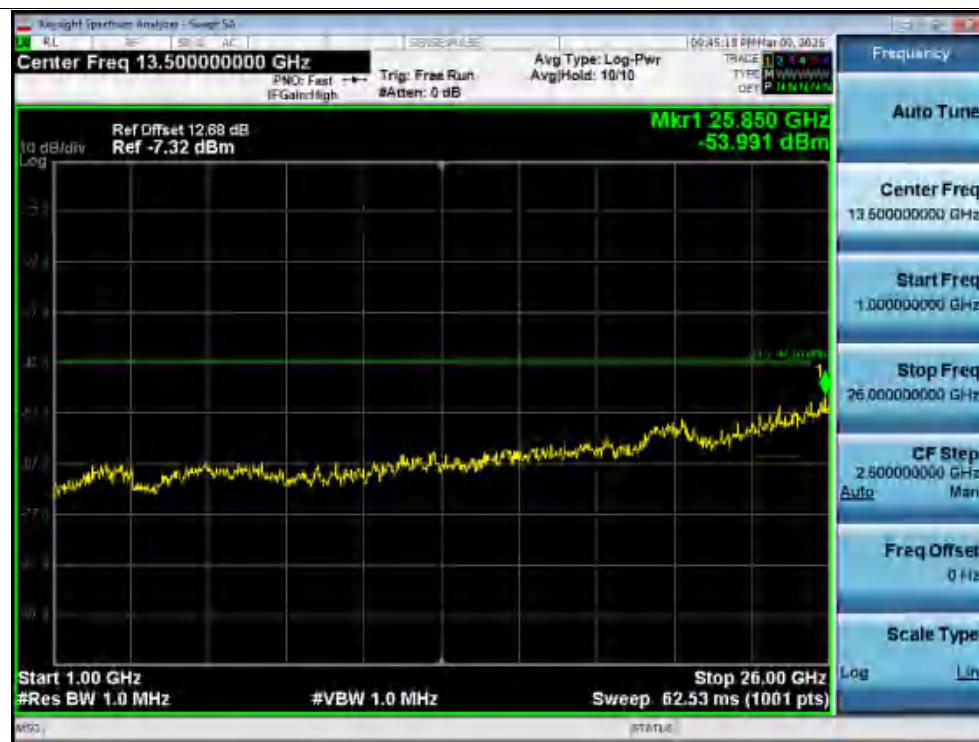
Rx. Spurious NVNT n40 5510MHz Ant1 @ 1000MHz-26000MHz
