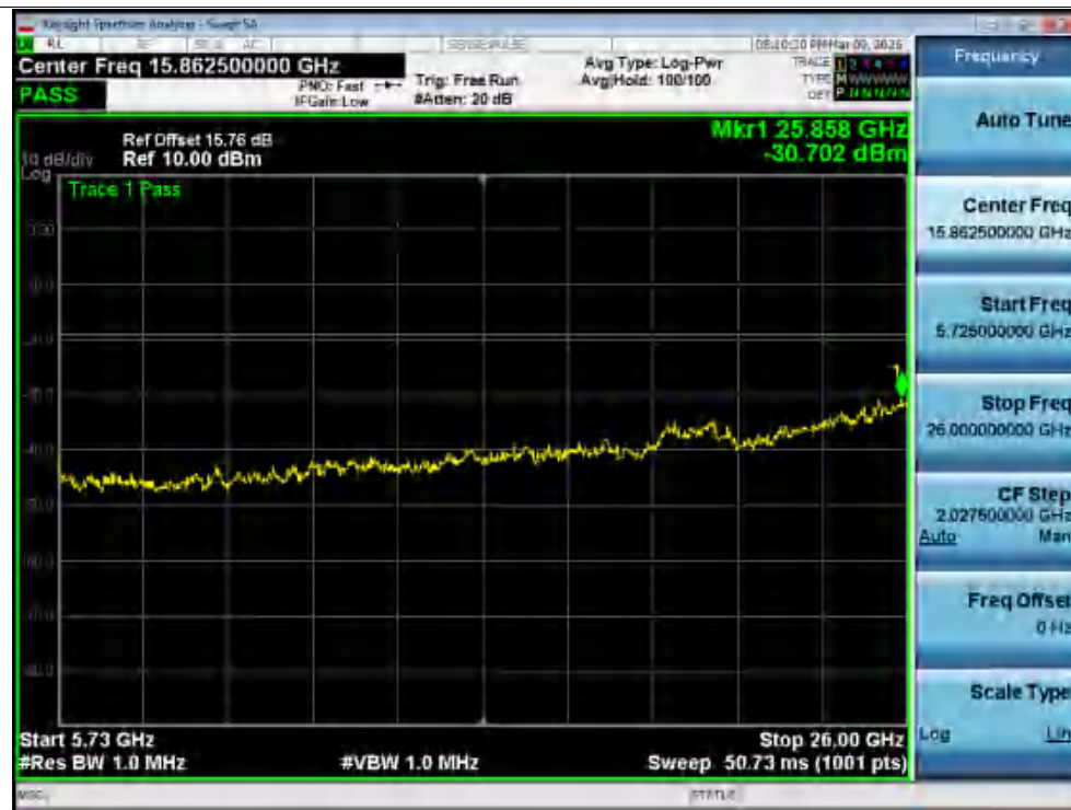
Tx. Spurious NVNT ax160 5570MHz Ant1 @ 30MHz-5419.6MHz
