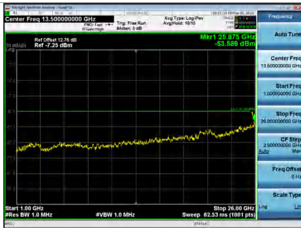
Rx. Spurious NVNT ac160 5570MHz Ant1 @ 1000MHz-26000MHz
