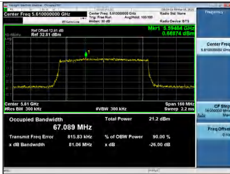
Spreading Bandwidth NVNT ax80 5610MHz Ant2
