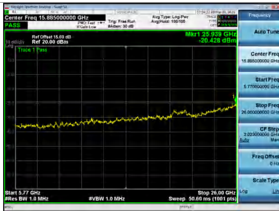
Tx. Spurious NVNT ac40 5510MHz Ant1 @ 5770MHz-26000MHz
