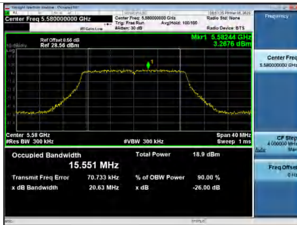
Spreading Bandwidth NVNT ac20 5580MHz Ant2
