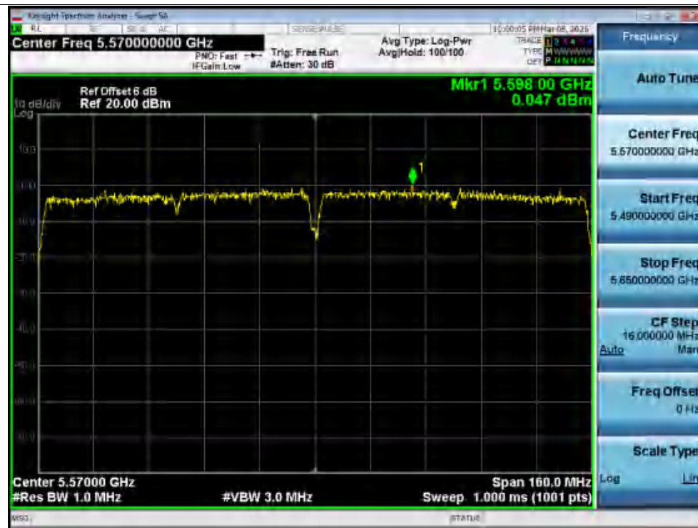
Power NVNT ac160 5570 MHz Ant2 Zero Span
