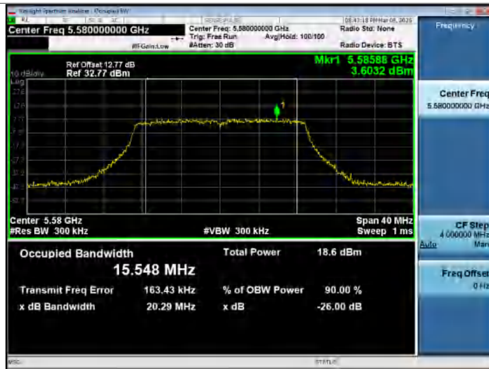
Spreading Bandwidth NVNT n20 5580MHz Ant2
