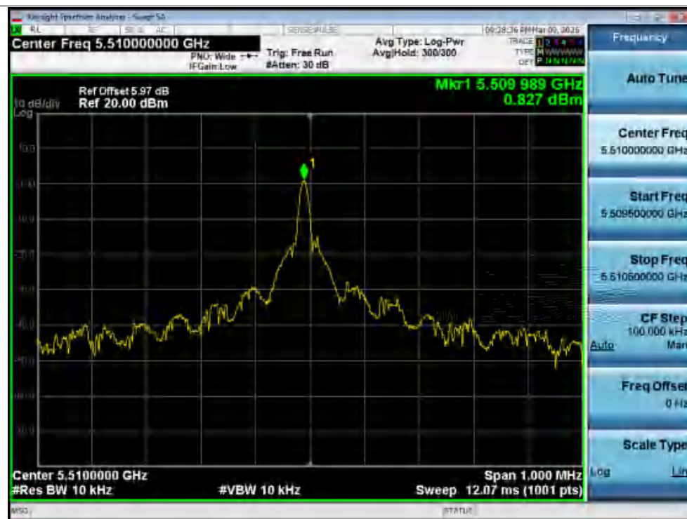
Freq. Error NVNT 5510MHz Ant2
