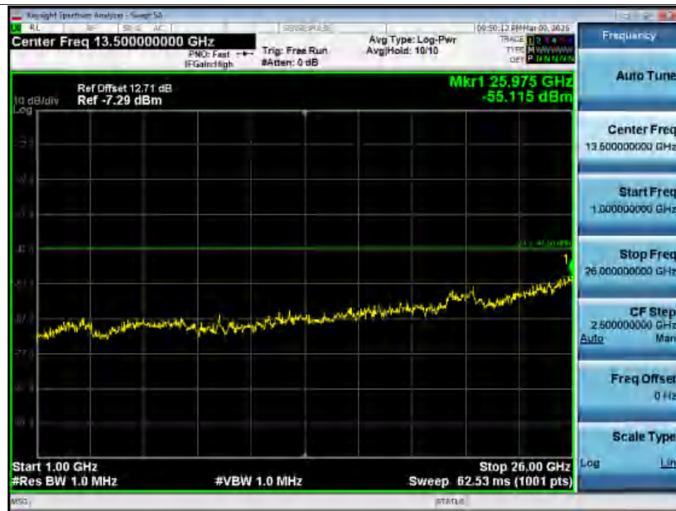
Rx. Spurious NVNT ax80 5530MHz Ant1 @ 1000MHz-26000MHz
