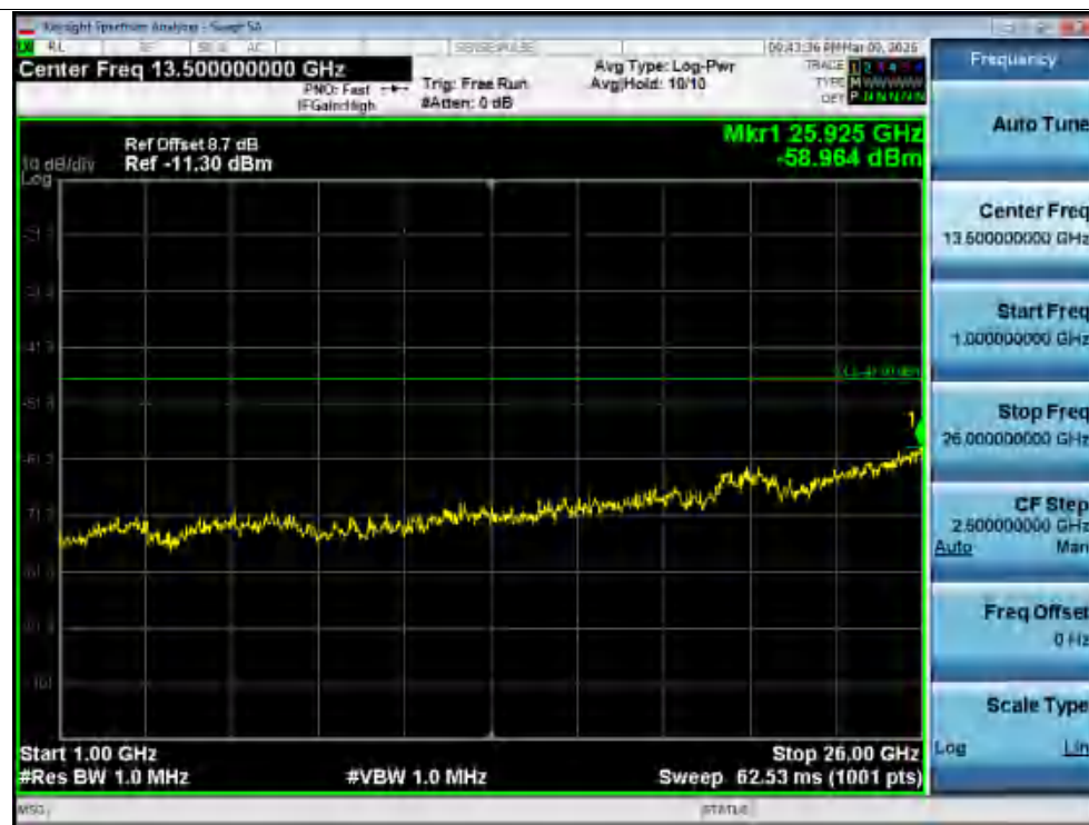
Rx. Spurious NVNT n20 5700MHz Ant2 @ 1000MHz-26000MHz
