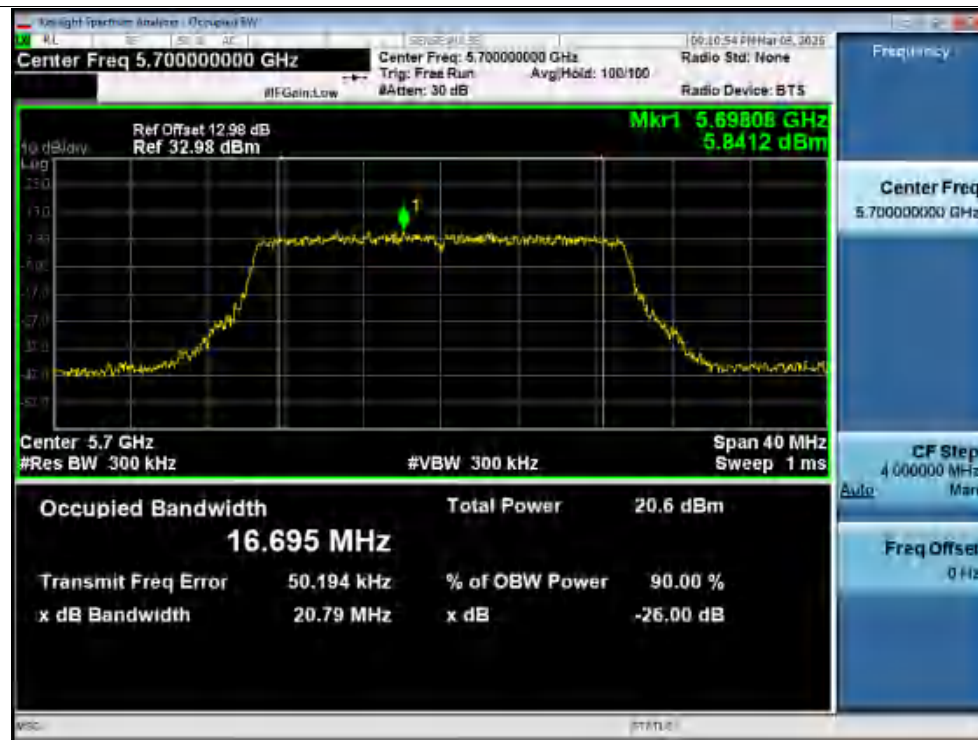
Spreading Bandwidth NVNT ax20 5700MHz Ant2
