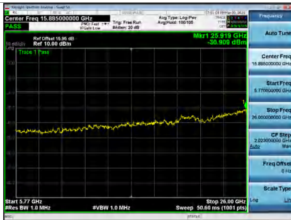
Tx. Spurious NVNT ac40 5670MHz Ant1 @ 5770MHz-26000MHz
