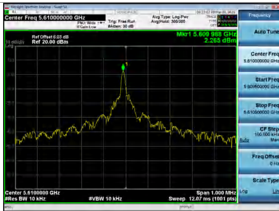
Freq. Error NVNT 5610MHz Ant2
