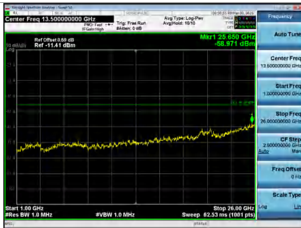
Rx. Spurious NVNT ac80 5610MHz Ant2 @ 1000MHz-26000MHz
