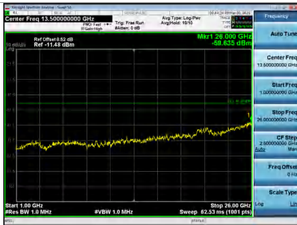
Rx. Spurious NVNT ax20 5500MHz Ant2 @ 1000MHz-26000MHz
