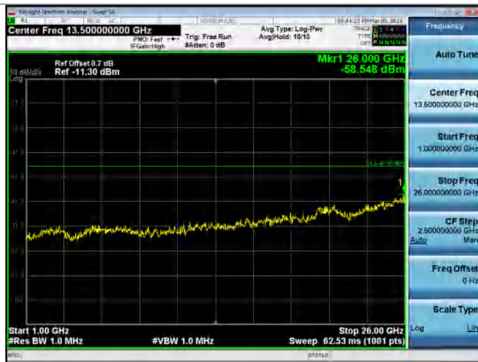
Rx. Spurious NVNT ac20 5700MHz Ant2 @ 1000MHz-26000MHz
