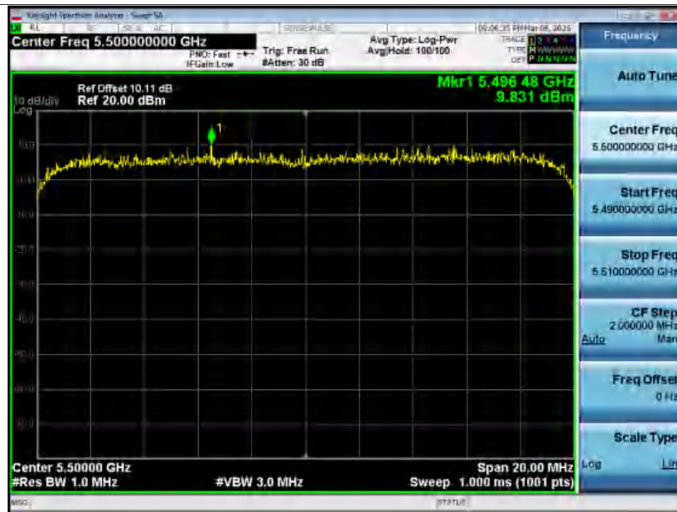
Power NVNT ax20 5500 MHz Ant1 Zero Span
