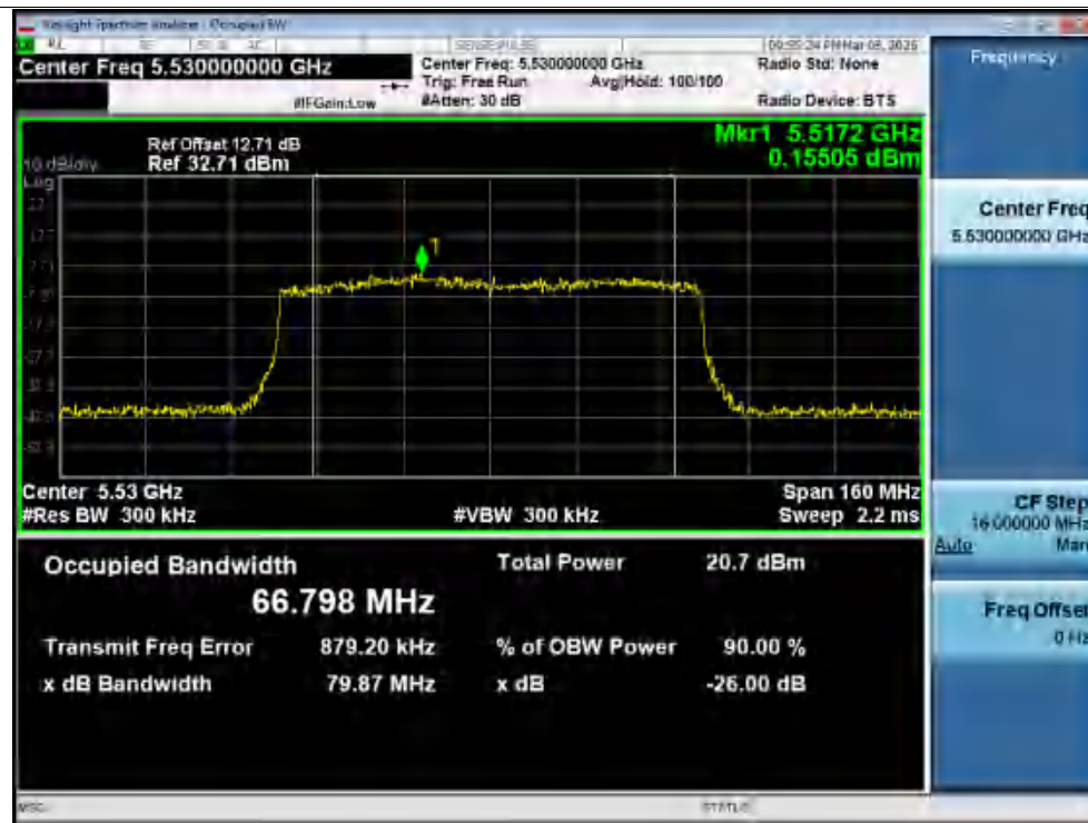
Spreading Bandwidth NVNT ax80 5530MHz Ant2
