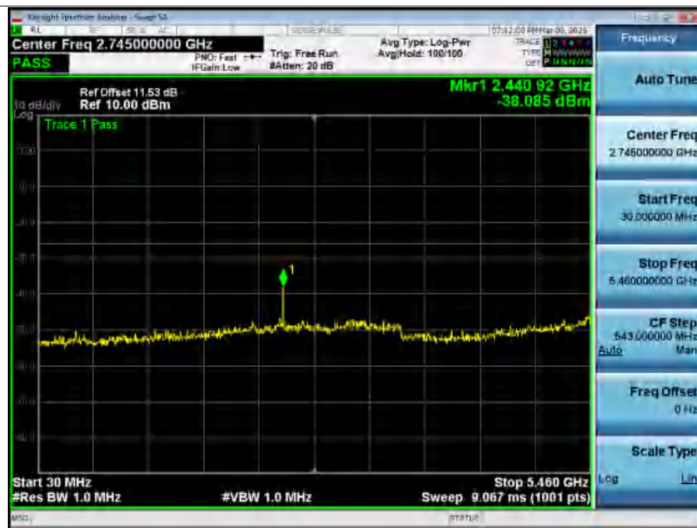
Tx. Spurious NVNT ac20 5500MHz Ant2 @ 30MHz-5460MHz
