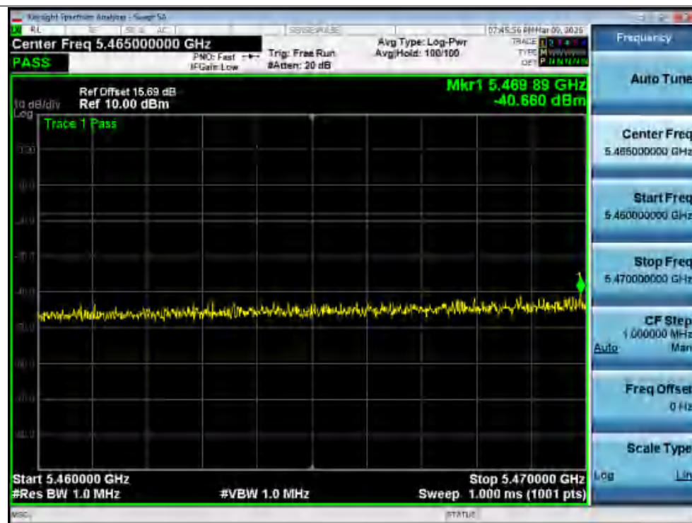
Tx. Spurious NVNT n40 5510MHz Ant1 @ 5460MHz-5470MHz
