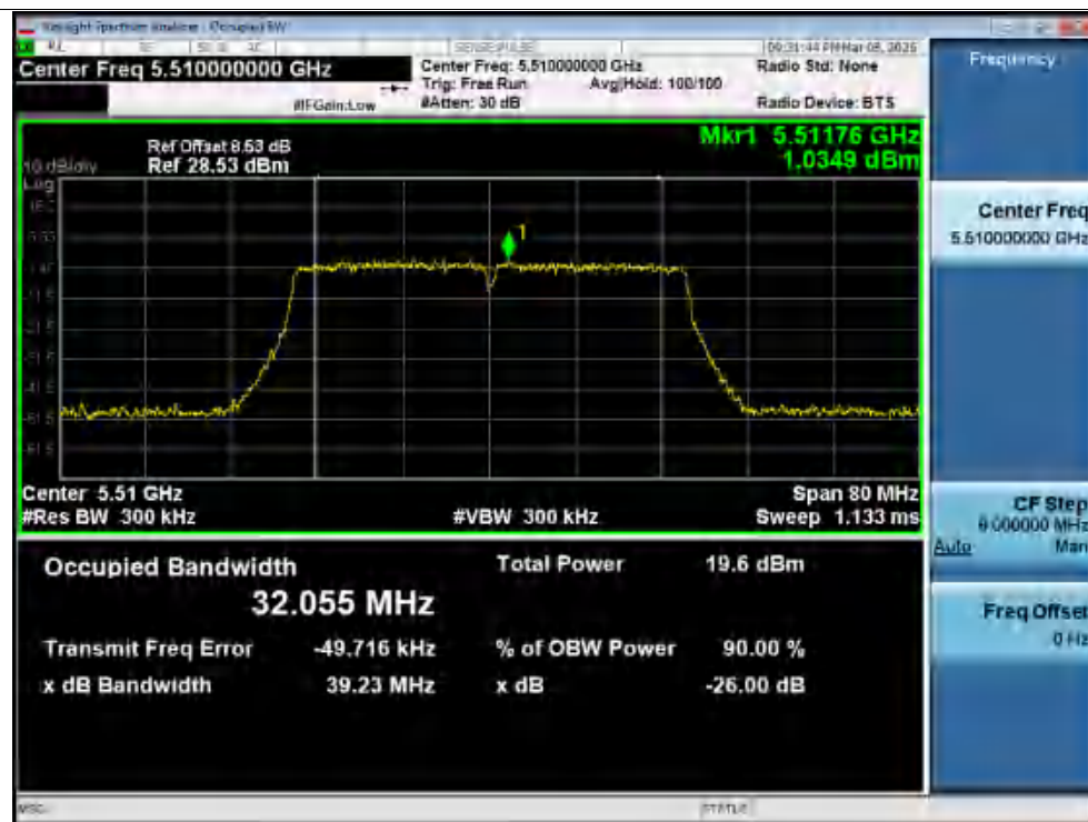
Spreading Bandwidth NVNT ac40 5510MHz Ant2
