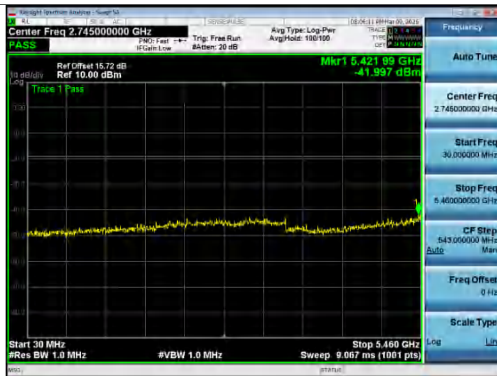
Tx. Spurious NVNT ax80 5530MHz Ant1 @ 30MHz-5460MHz
