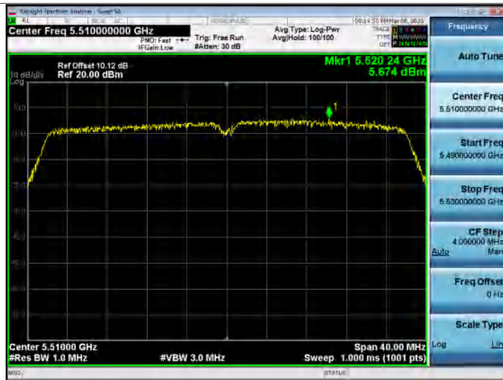
Power NVNT n40 5510 MHz Ant1 Zero Span
