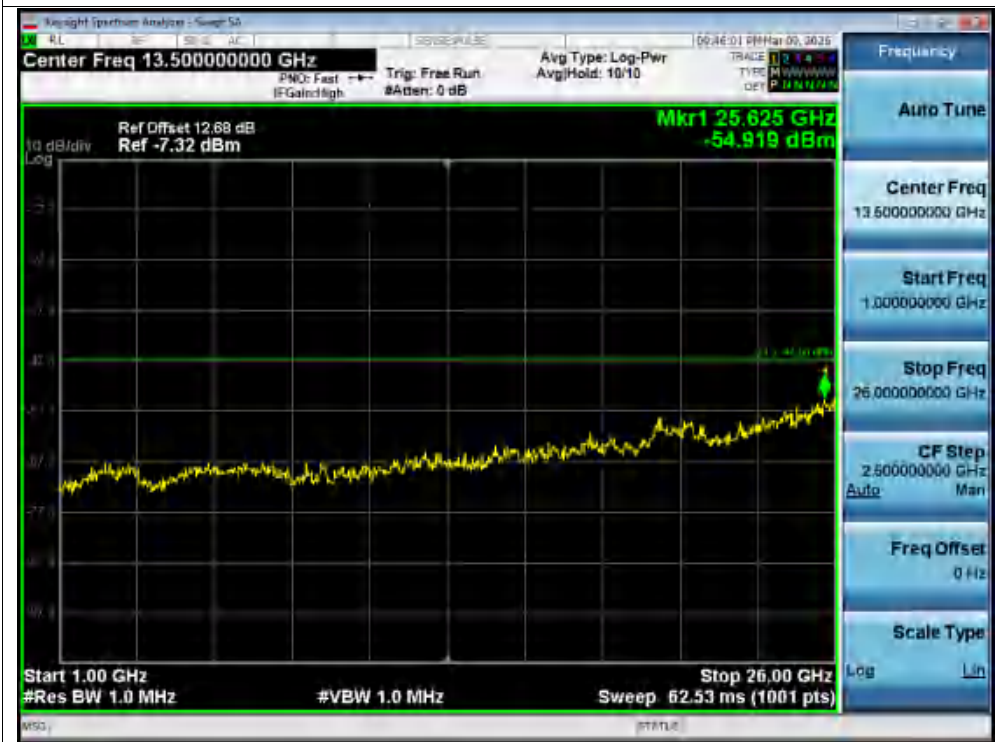
Rx. Spurious NVNT ac40 5510MHz Ant1 @ 1000MHz-26000MHz
