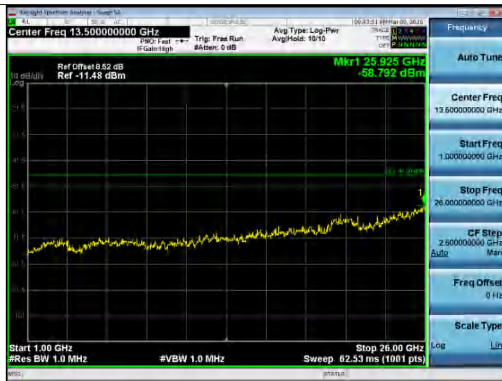
Rx. Spurious NVNT ac20 5500MHz Ant2 @ 1000MHz-26000MHz
