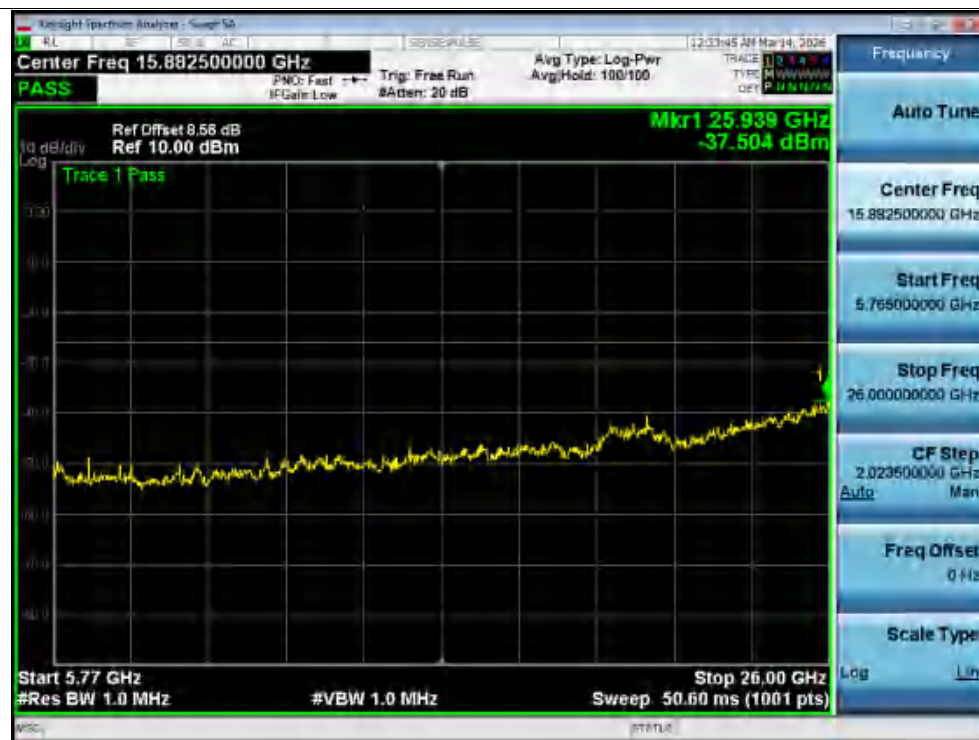
Tx. Spurious NVNT a 5580MHz Ant2 @ 5765MHz-26000MHz
