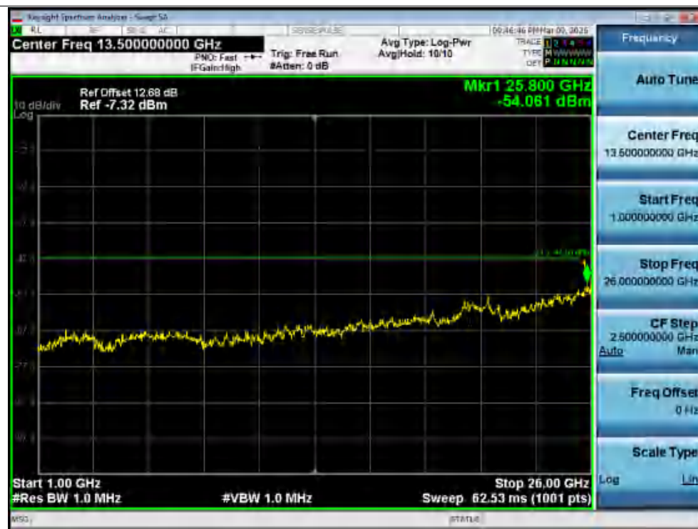
Rx. Spurious NVNT ax40 5510MHz Ant1 @ 1000MHz-26000MHz
