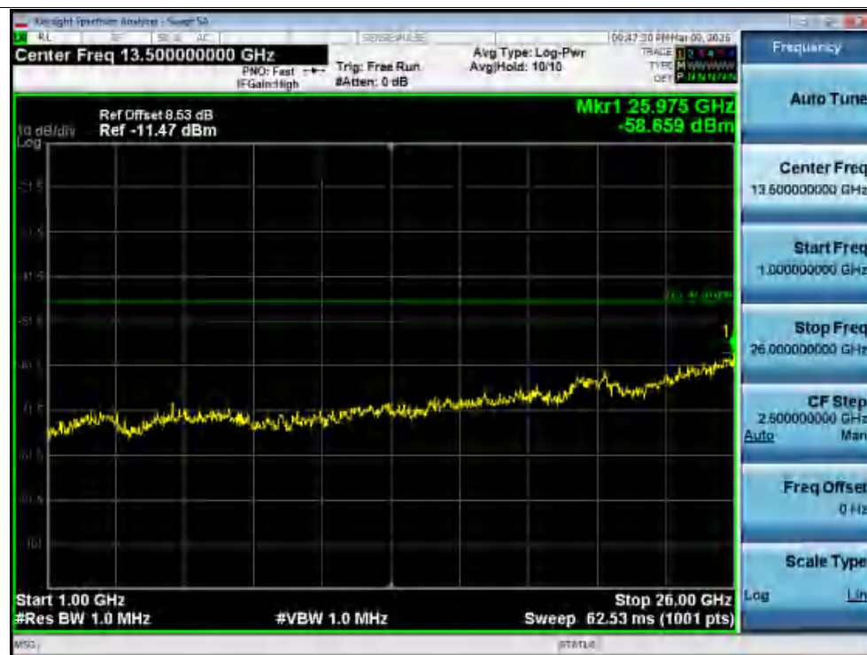
Rx. Spurious NVNT n40 5510MHz Ant2 @ 1000MHz-26000MHz
