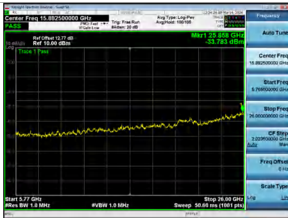
Tx. Spurious NVNT a 5580MHz Ant1 @ 5765MHz-26000MHz
