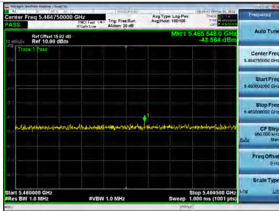
Tx. Spurious NVNT ax80 5610MHz Ant1 @ 5469.5MHz-5470MHz
