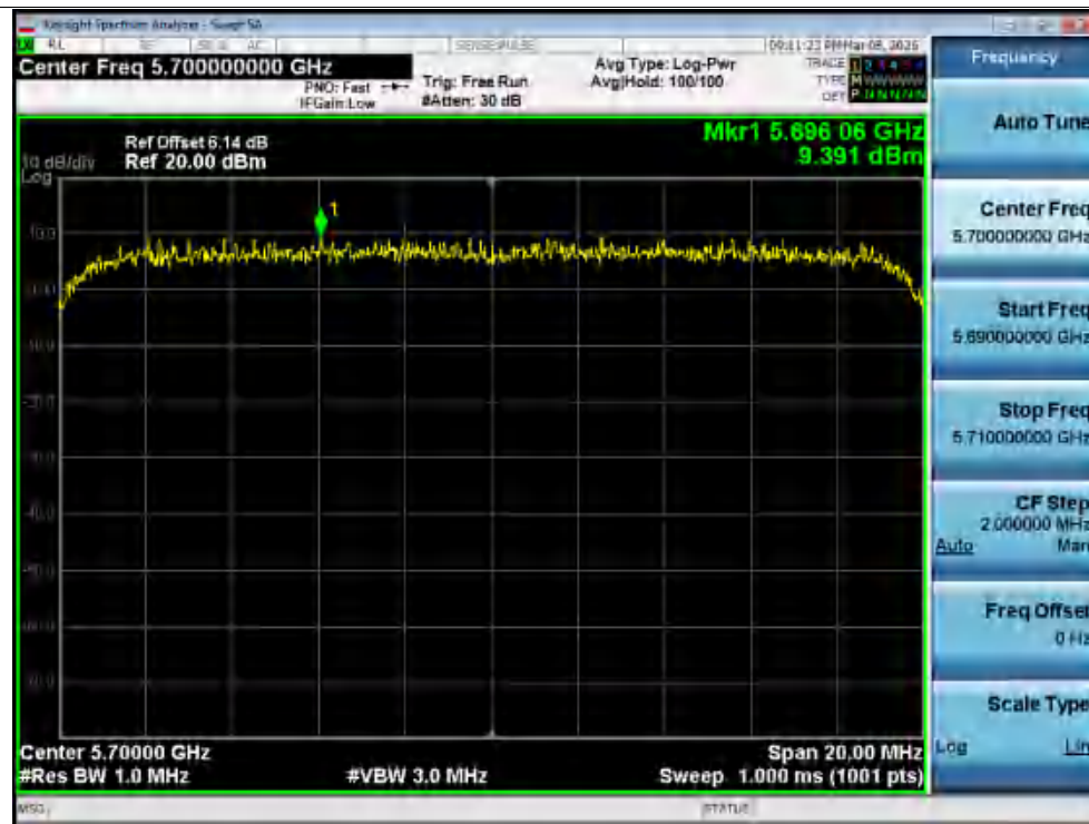
Power NVNT ax20 5700 MHz Ant2 Zero Span
