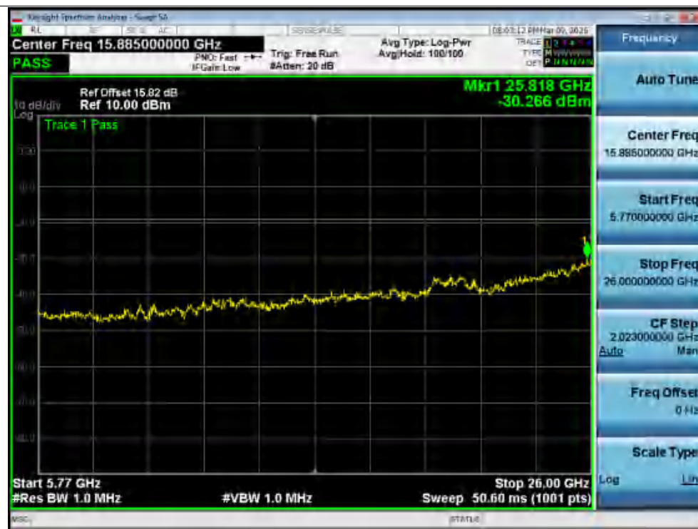
Tx. Spurious NVNT ac80 5610MHz Ant1 @ 5770MHz-26000MHz
