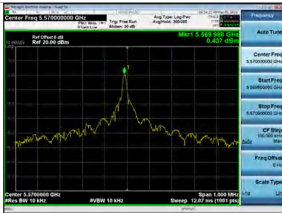
Freq. Error NVNT 5570MHz Ant2
