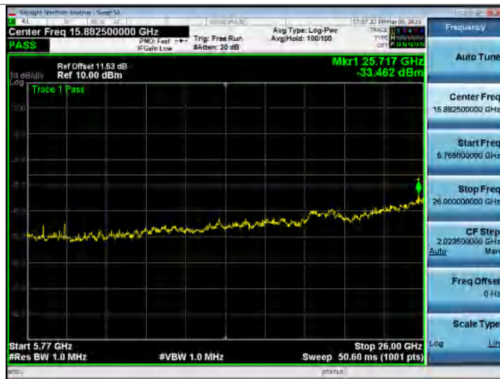
Tx. Spurious NVNT ax20 5500MHz Ant2 @ 5765MHz-26000MHz
