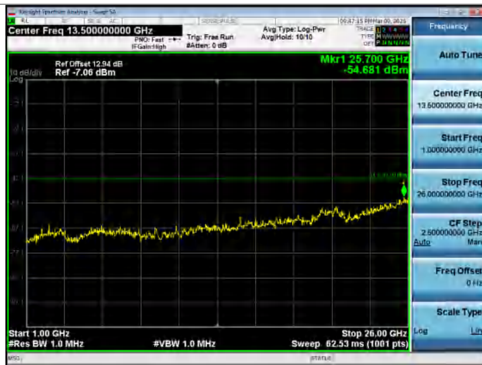
Rx. Spurious NVNT ax40 5670MHz Ant1 @ 1000MHz-26000MHz
