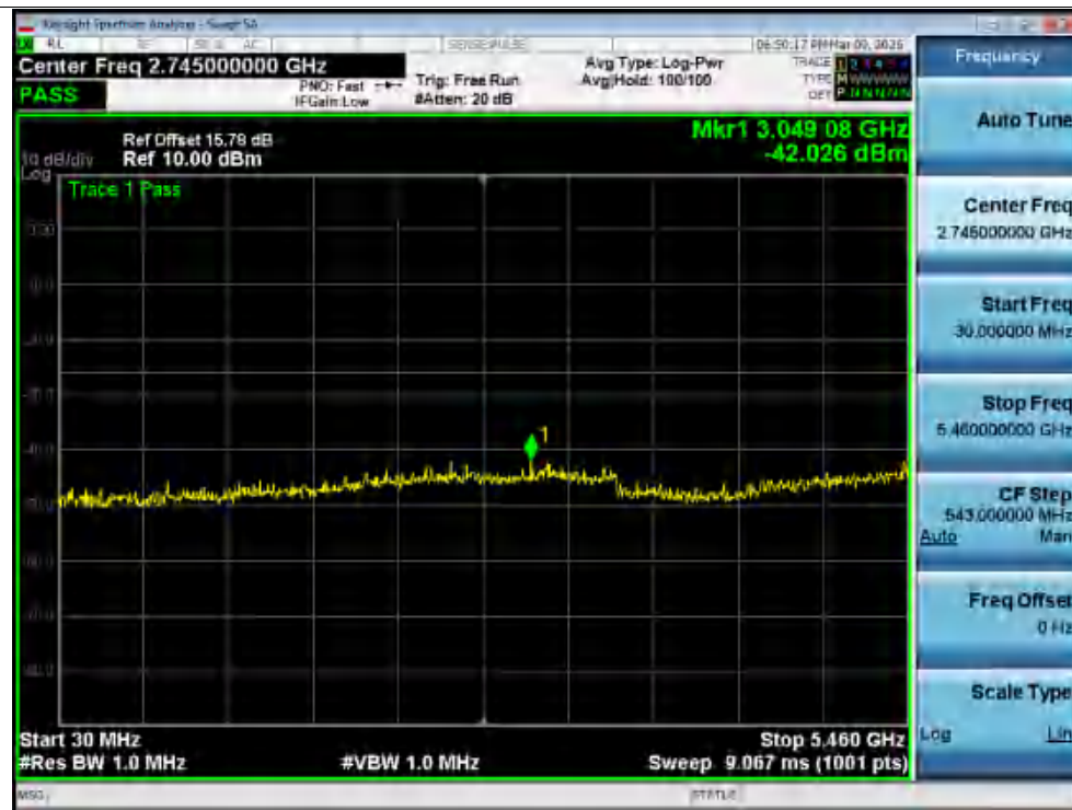
Tx. Spurious NVNT n20 5580MHz Ant1 @ 5460MHz-5470MHz
