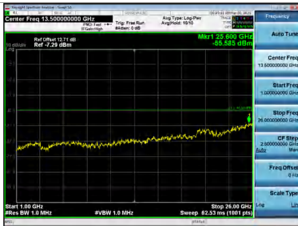
Rx. Spurious NVNT ac80 5530MHz Ant1 @ 1000MHz-26000MHz
