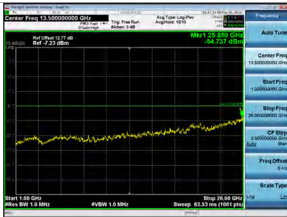
Rx. Spurious NVNT ac20 5580MHz Ant1 @ 1000MHz-26000MHz
