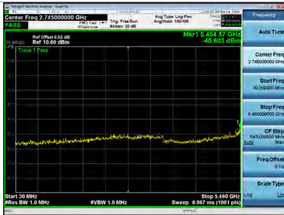
Tx. Spurious NVNT a 5500MHz Ant2 @ 5460MHz-5470MHz
