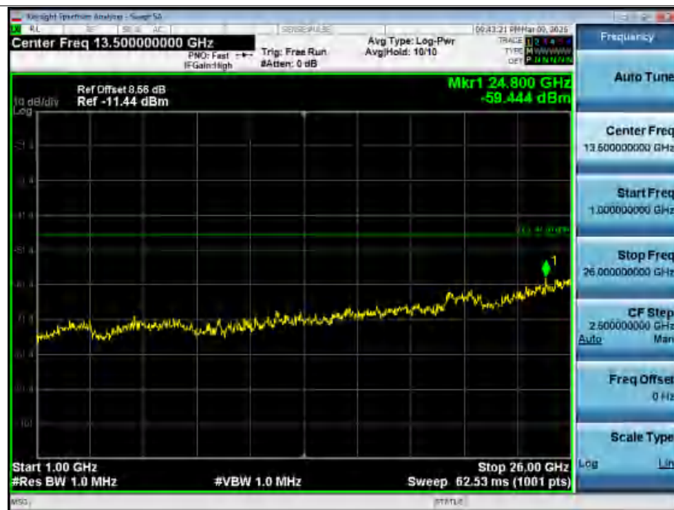
Rx. Spurious NVNT n20 5580MHz Ant2 @ 1000MHz-26000MHz
