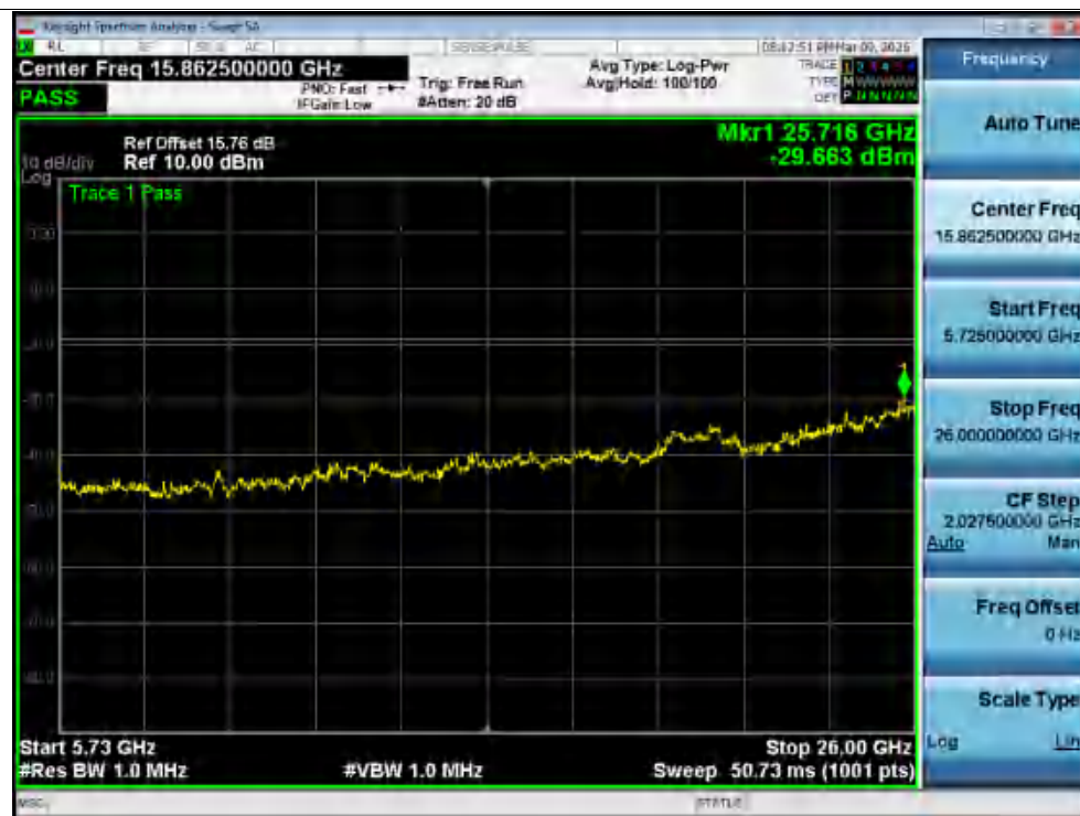
Tx. Spurious NVNT ax160 5570MHz Ant1 @ 5725MHz-26000MHz
