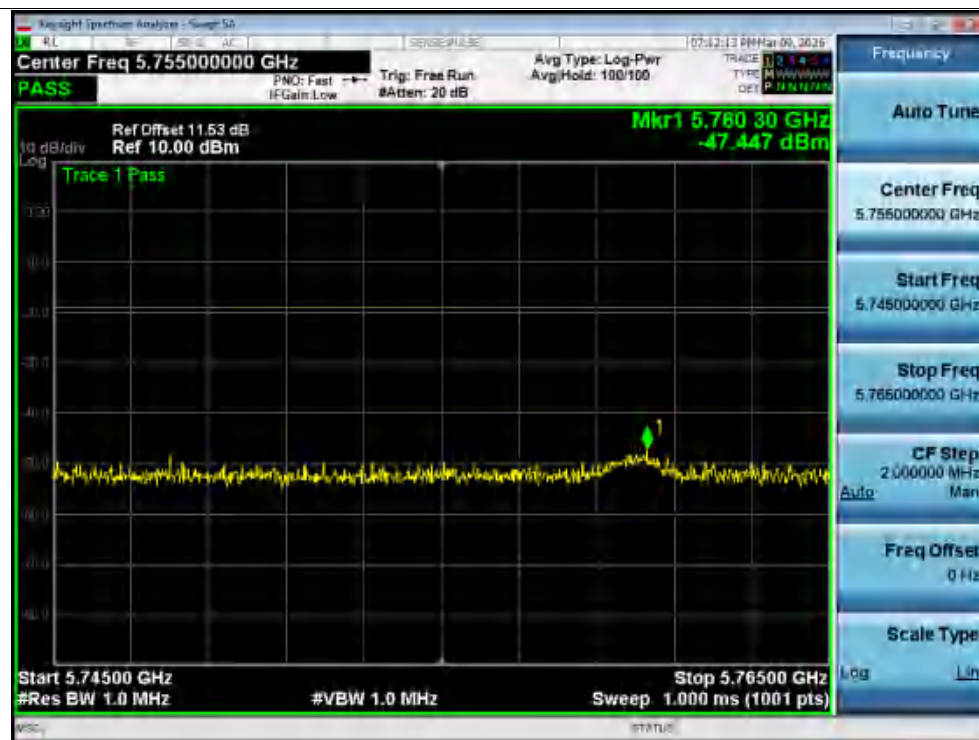
Tx. Spurious NVNT ac20 5500MHz Ant2 @ 5745MHz-5765MHz
