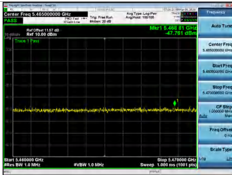
Tx. Spurious NVNT ac20 5580MHz Ant2 @ 5745MHz-5765MHz
