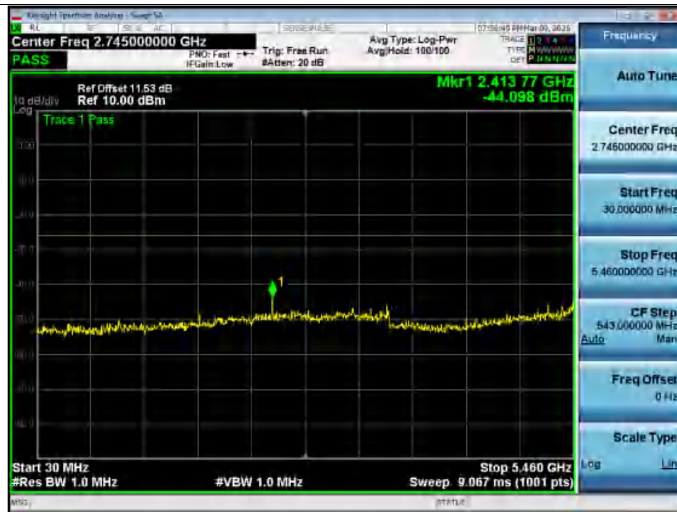
Tx. Spurious NVNT ax20 5500MHz Ant2 @ 5460MHz-5470MHz
