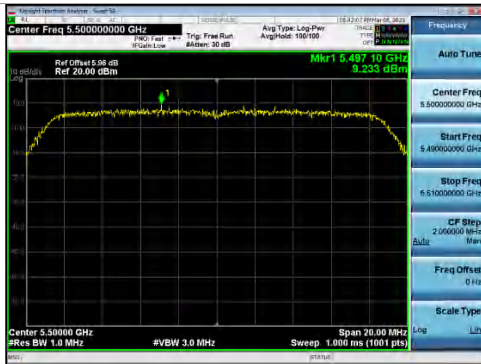
Power NVNT n20 5500 MHz Ant2 Zero Span
