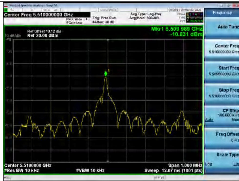
Freq. Error NVNT 5590MHz Ant1
