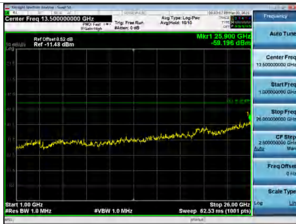
Rx. Spurious NVNT n20 5500MHz Ant2 @ 1000MHz-26000MHz
