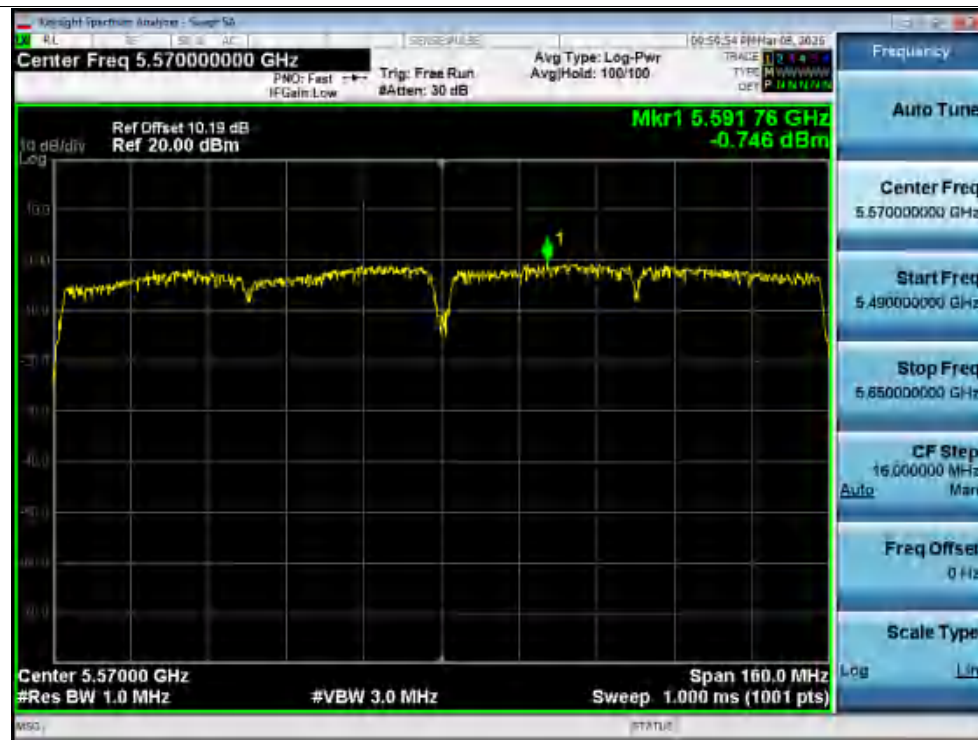
Power NVNT ac160 5570 MHz Ant1 Zero Span
