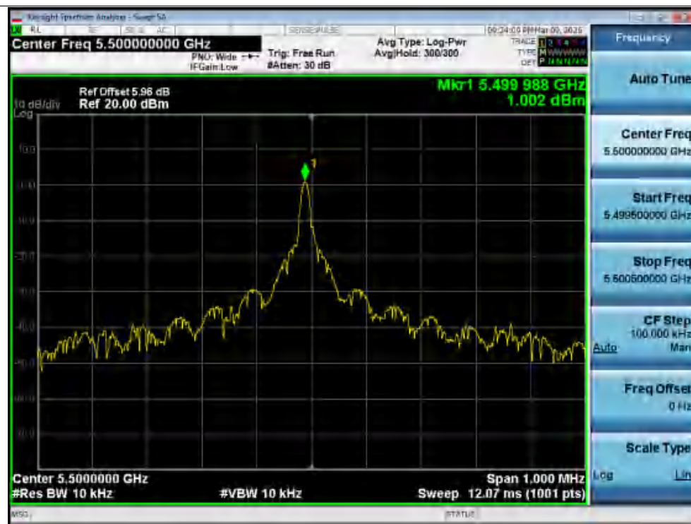
Freq. Error NVNT 5500MHz Ant2
