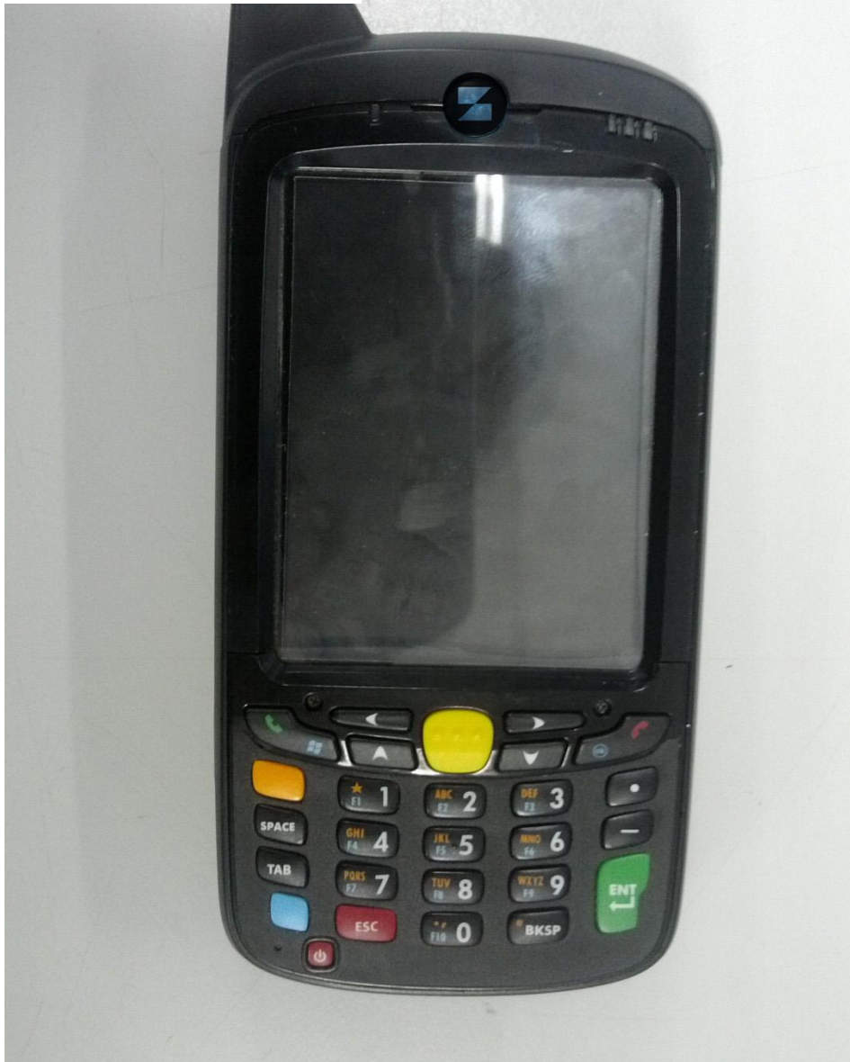
Numeric_DSD Keypad without Camera
