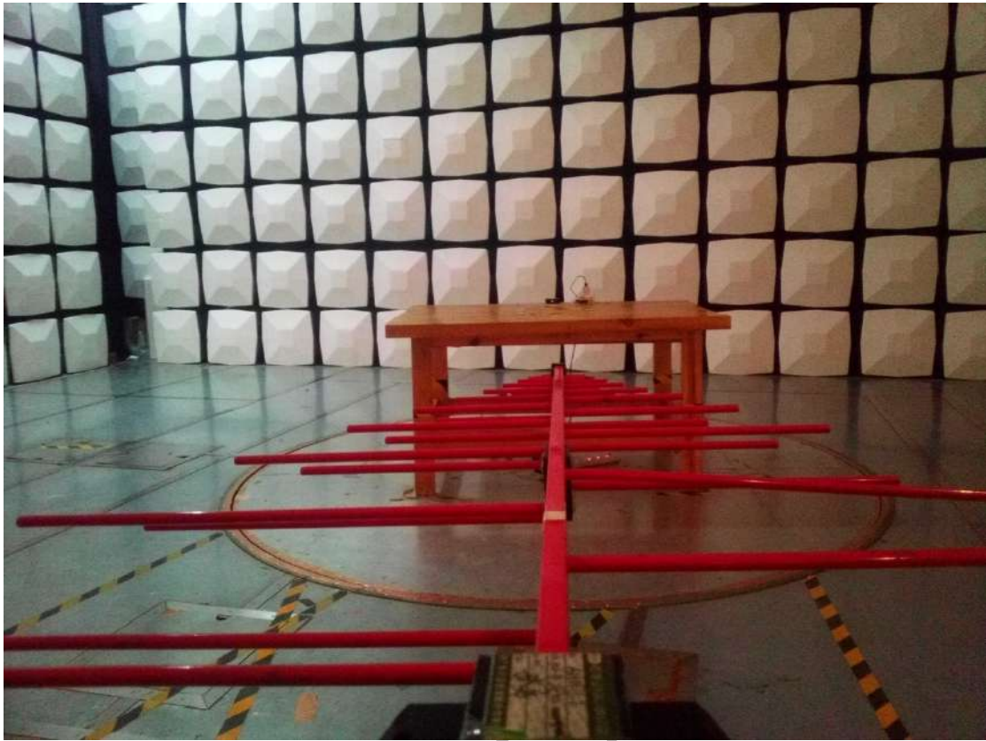
RE Below 1G front View
