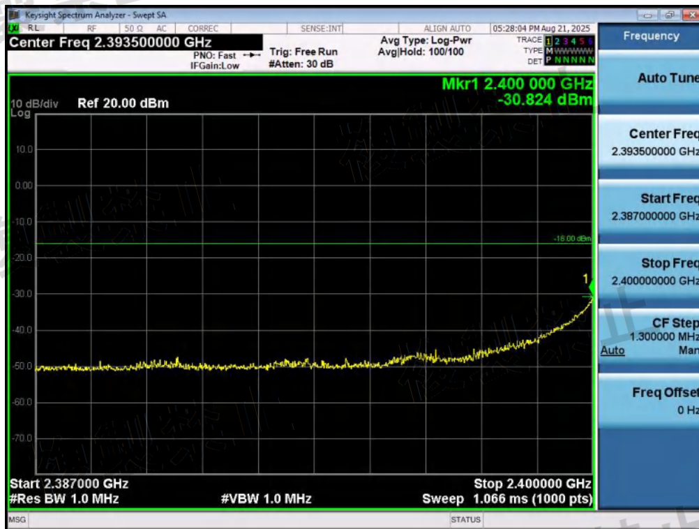
Test Graph BR ANT1 2402 1Mbps 2387 2400MHz NV
