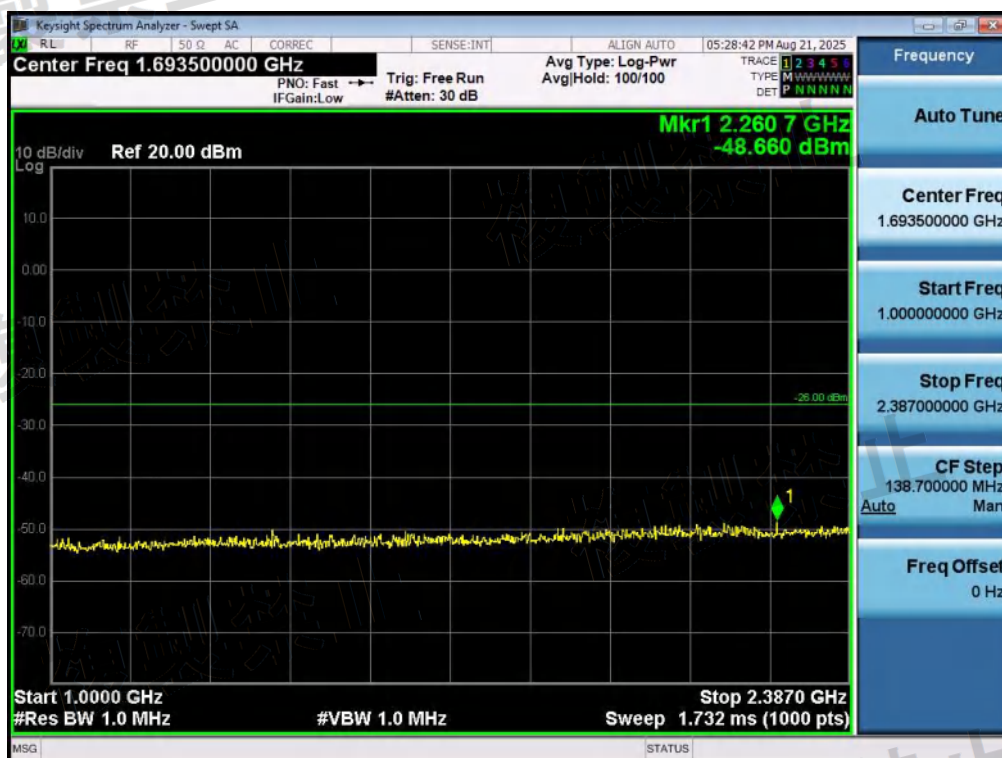
Test Graph BR ANT1 2402 1Mbps 1000 2387MHz LV
