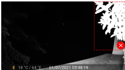
Figure 11: Avoid close-up obstacles in front of the camera
