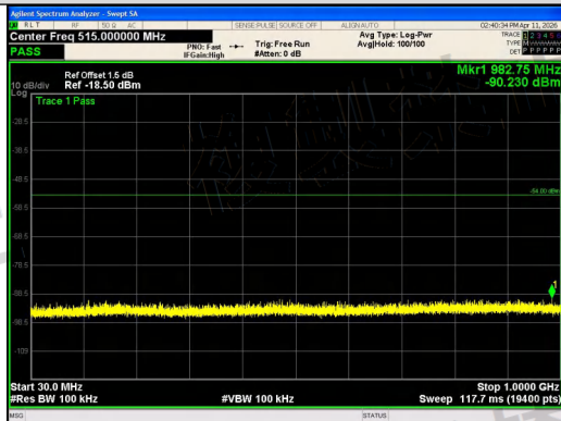
30MHz - 1000MHz NT/NV_Total_IEEE 802.11ax_80_Channel 106_RU&Index SU
