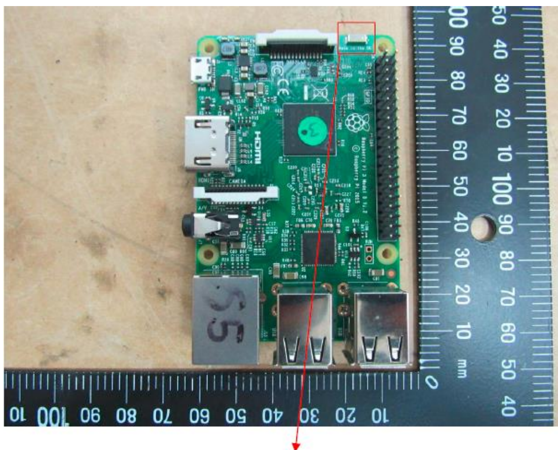
Chip Antenna / 1.87149 dBi
