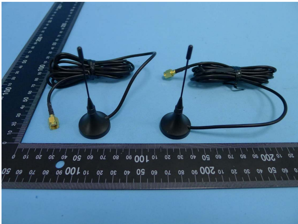
(4) 待測物照片 (External Antenna List (outdoor) / 4YA1260-1393 )
