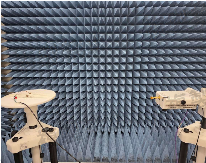
Radiated Measurement Photo 90 - 135 GHz
