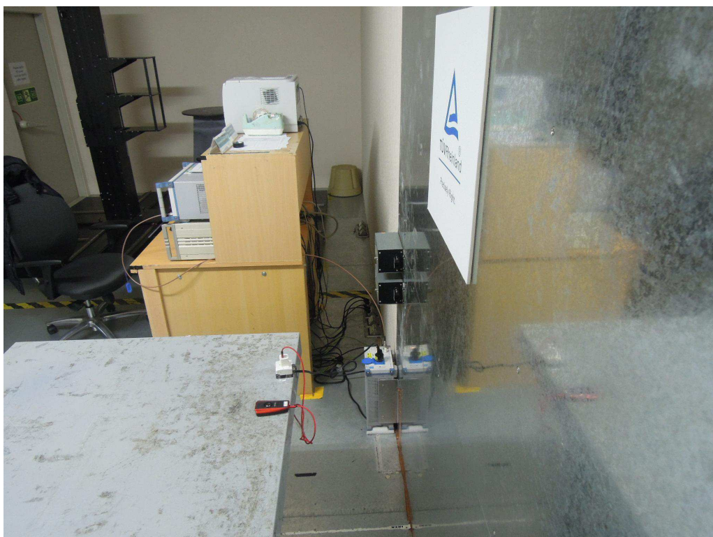
Photograph 9: Set-up for Mains Conducted testing Back
