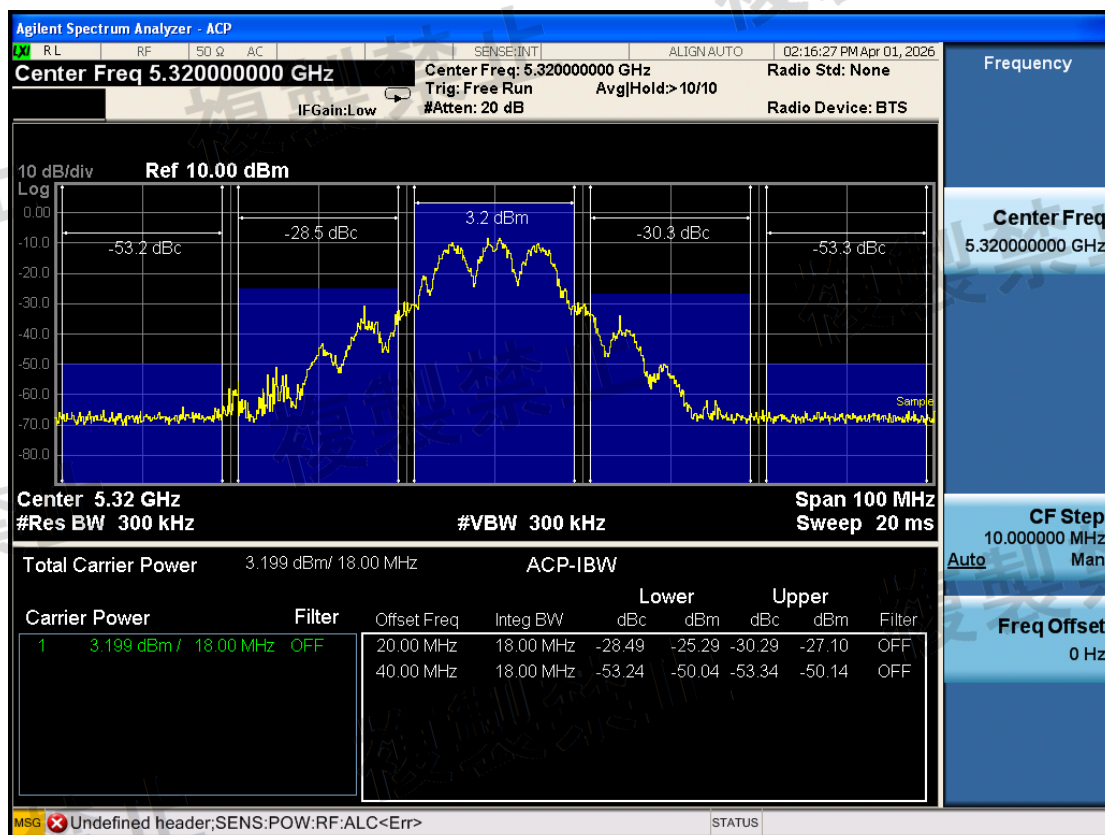
W53\Adjacent Channel Leakage Power\802.11a\5320-X-N
