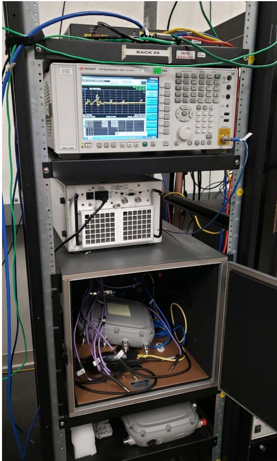
Title: Radio Conducted Test Setup – Rack 9
