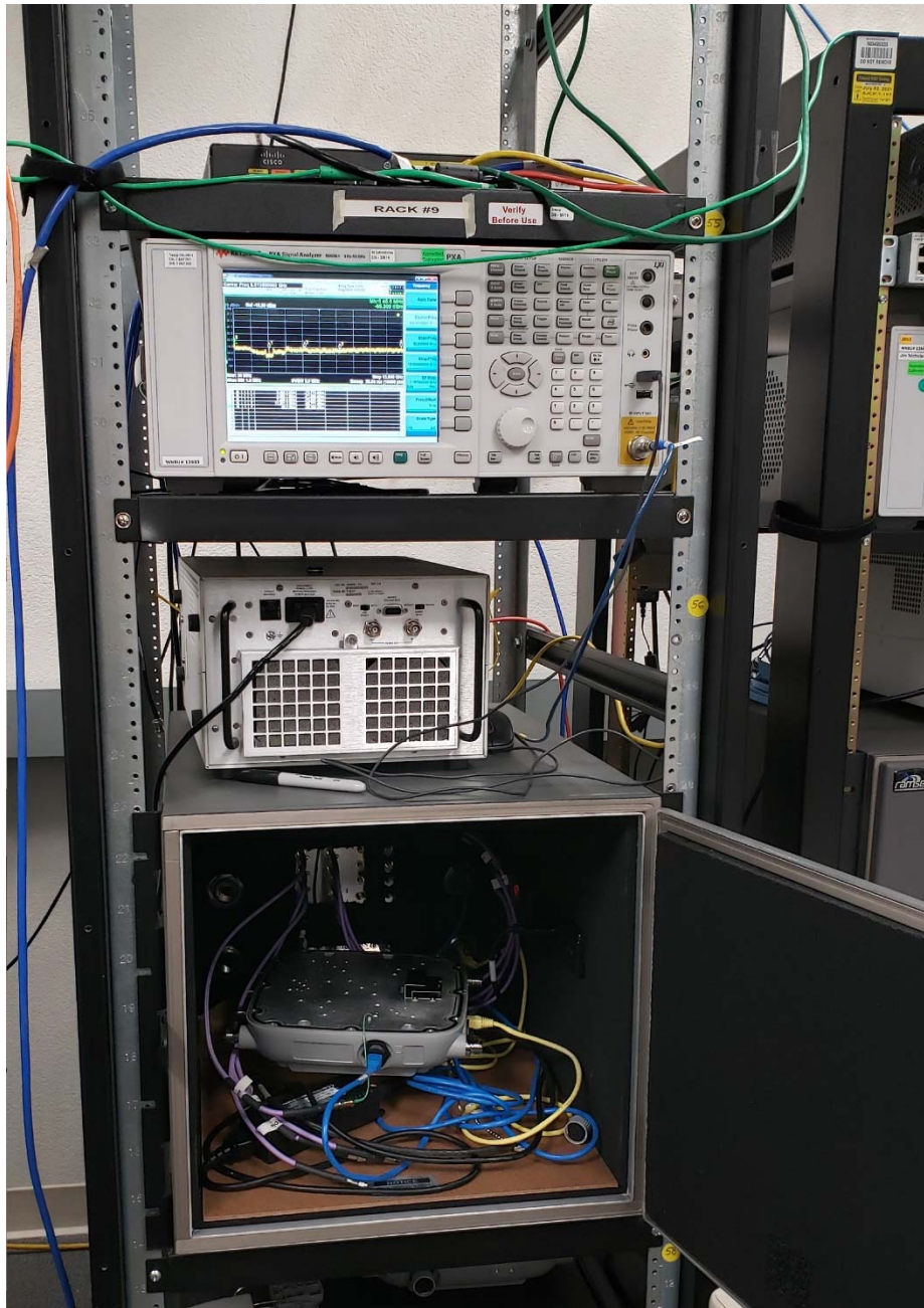
Title: Radio Conducted Test Setup – Rack 4 – BLE
