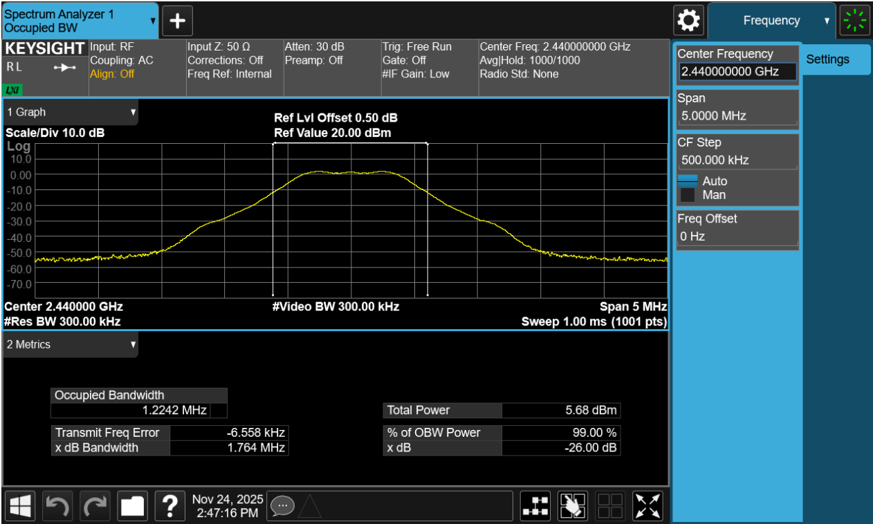
Figure 8-Occupied Bandwidth of 2440MHz
