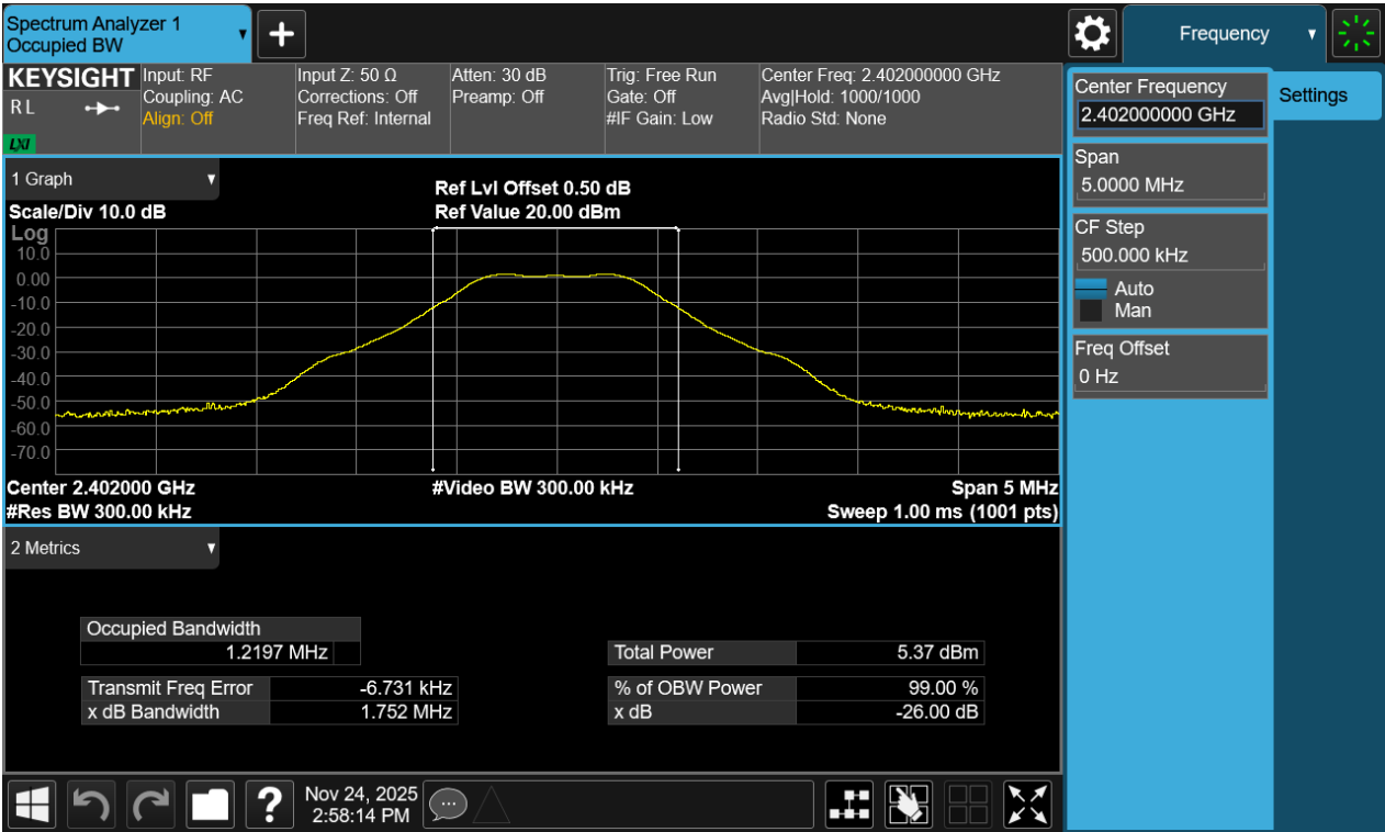
Figure 10-Occupied Bandwidth of 2402MHz
