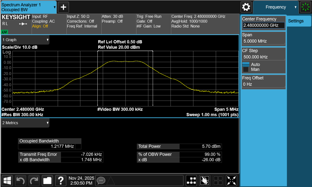
Figure 9-Occupied Bandwidth of 2480MHz
