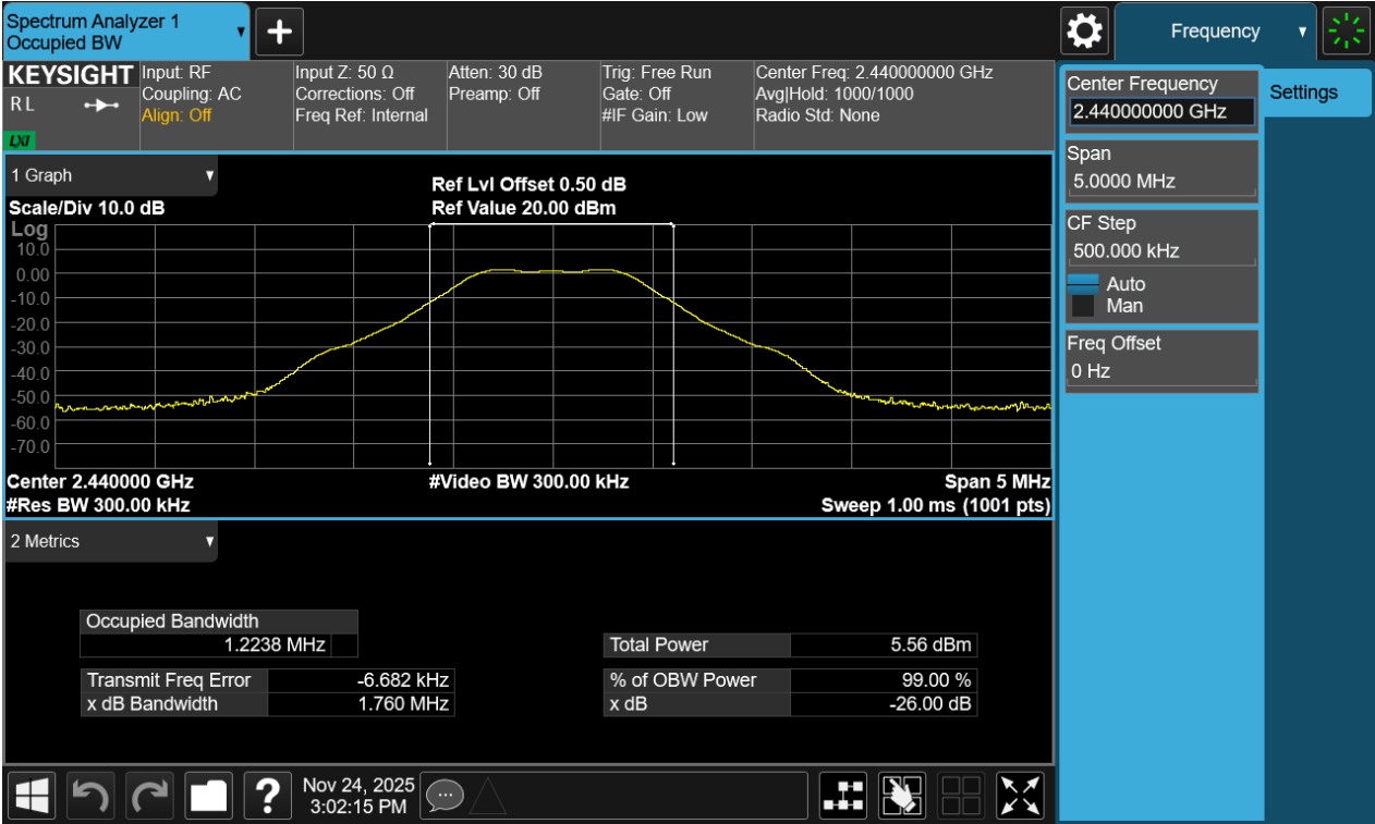
Figure 11-Occupied Bandwidth of 2440MHz
