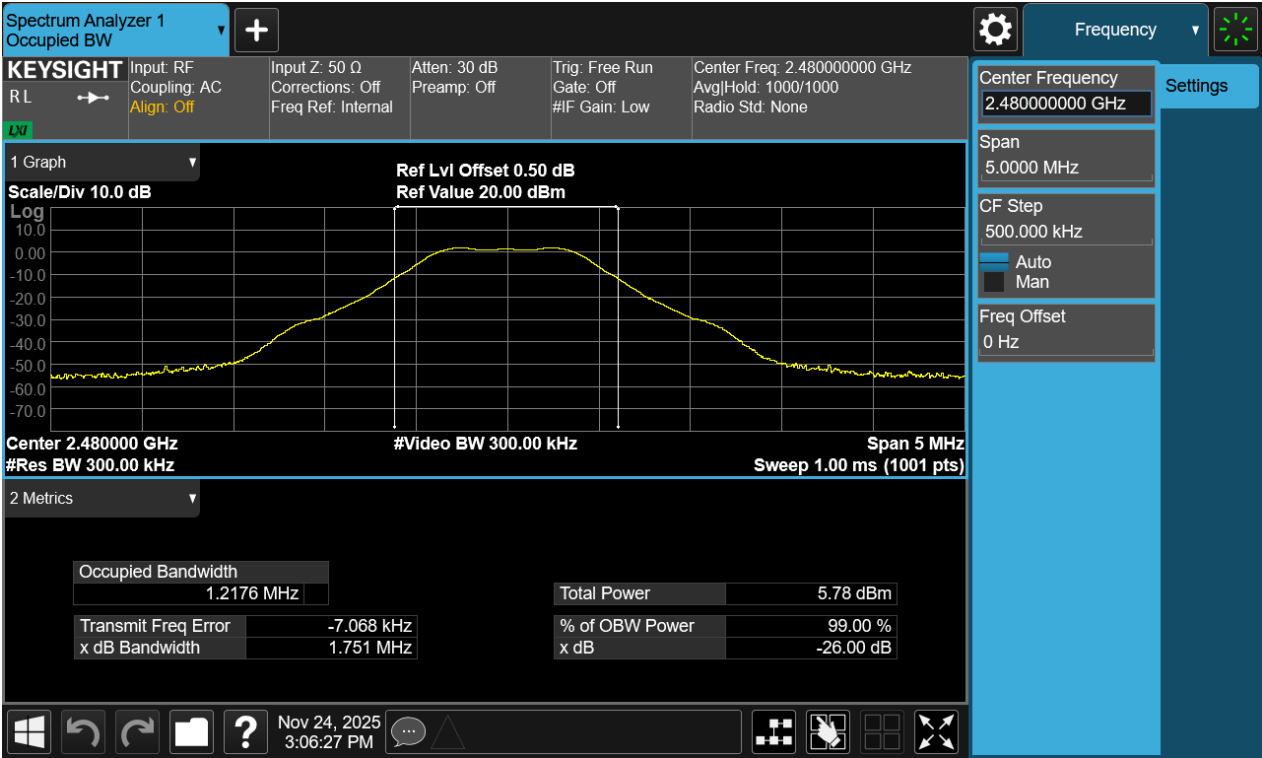
Figure 12-Occupied Bandwidth of 2480MHz
