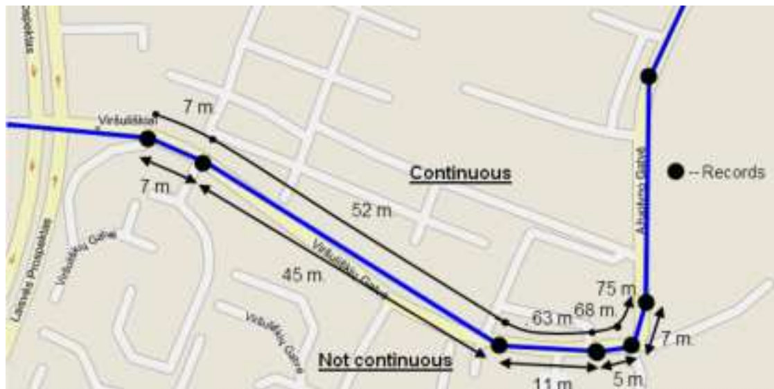
Figure 20 Trip continuous distance counting parameter example
