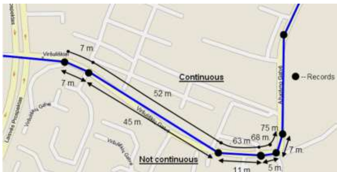
Figure 9 Odometer continuous and Not continuous distance counting parameter example
