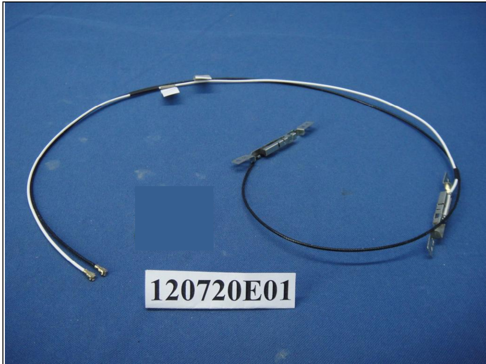
Antenna 2: Brand : WNC / Model : 81.ED415.001 (For WLAN & BT Used)
