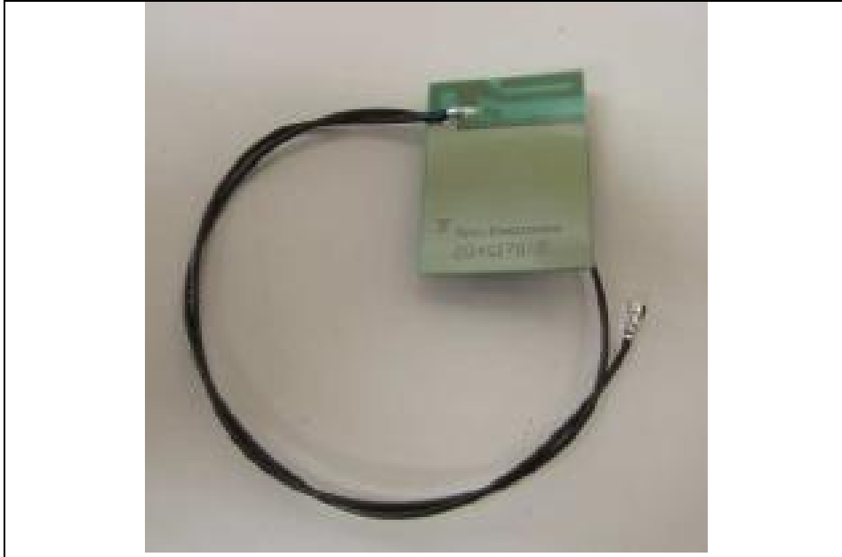
Antenna 16: Brand : Tyco / Model : TBN005 (TX1) / TBN005 (TX2) (For WLAN & BT Used)
