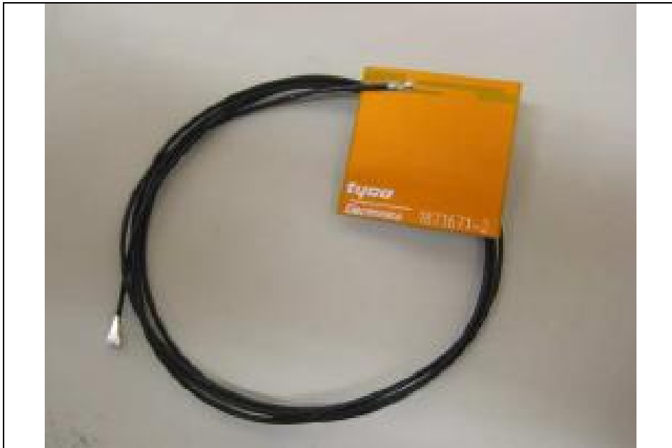
Antenna 15: Brand : Tyco / Model : TBN001 (TX1) / TBN001 (TX2) (For WLAN & BT Used)
