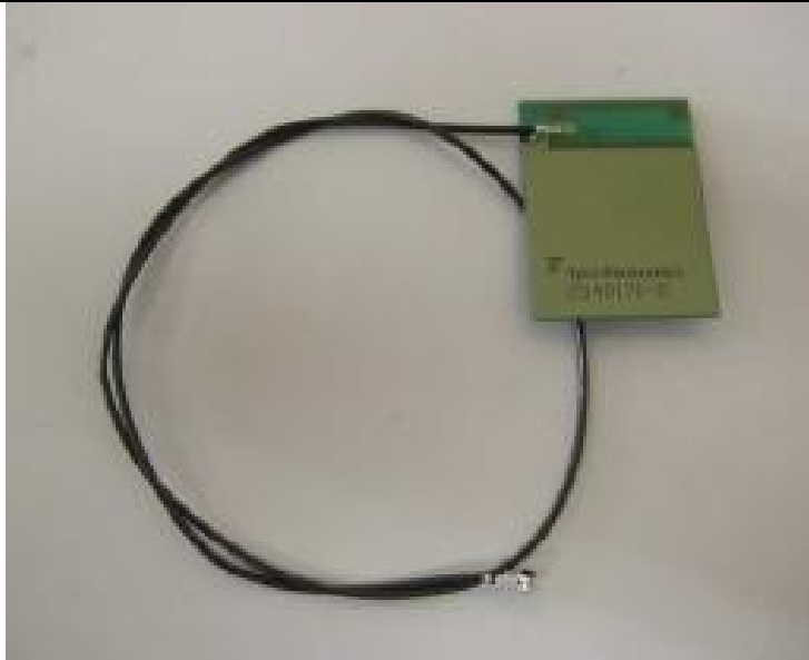
Antenna 17: Brand : Tyco / Model : TBN006 (TX1) / TBN006 (TX2) (For WLAN & BT Used)
