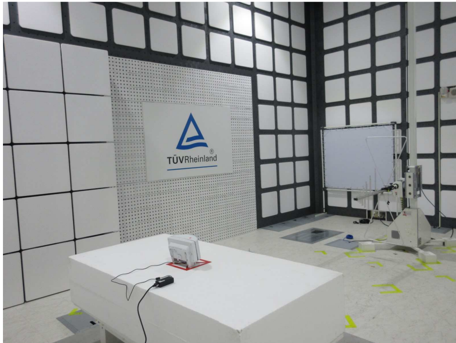
Photograph 3: Set-up for Spurious Emissions (Back View 1)
