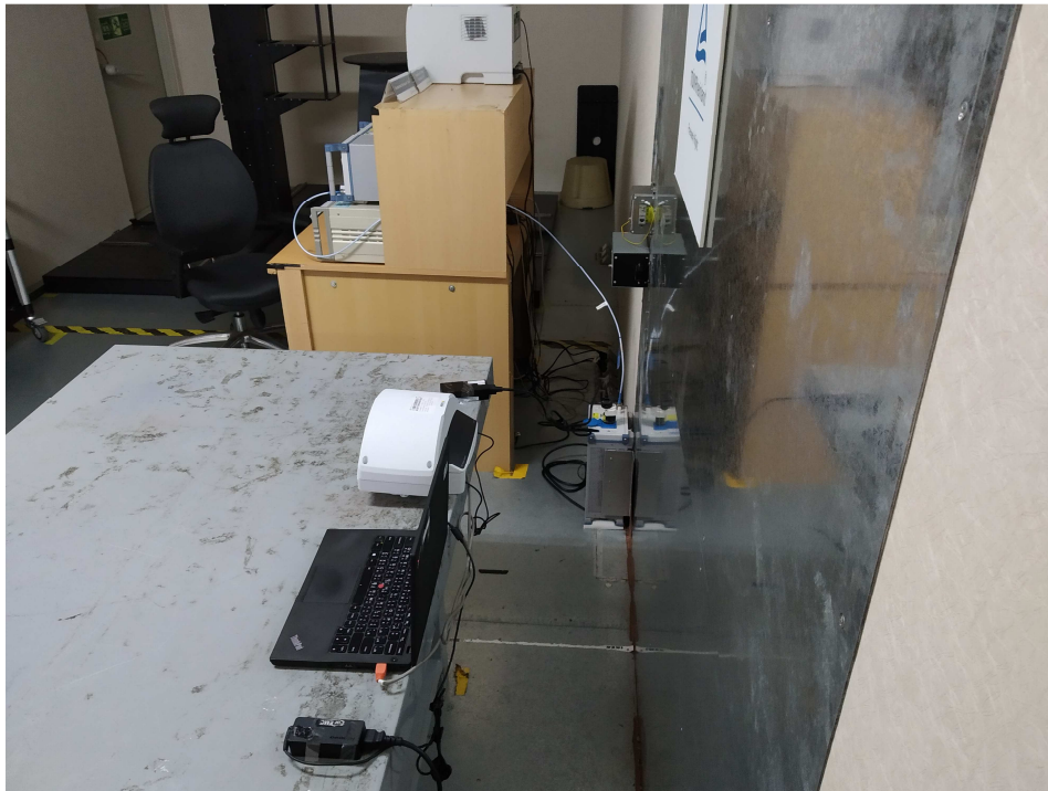
Photograph 7: Set-up for for Mains Conducted testing Back
