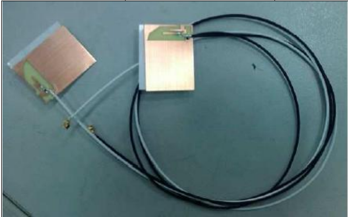
PIFA Antenna (Brand name: ACON, Model No.: ACTA-02)
