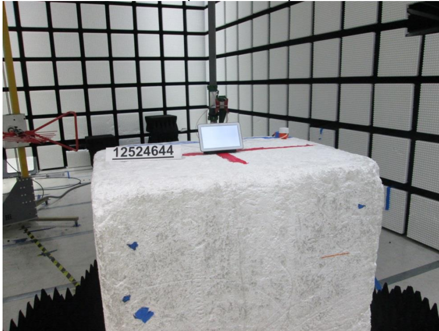
RADIATED BACK PHOTO (ABOVE 1 GHz)
