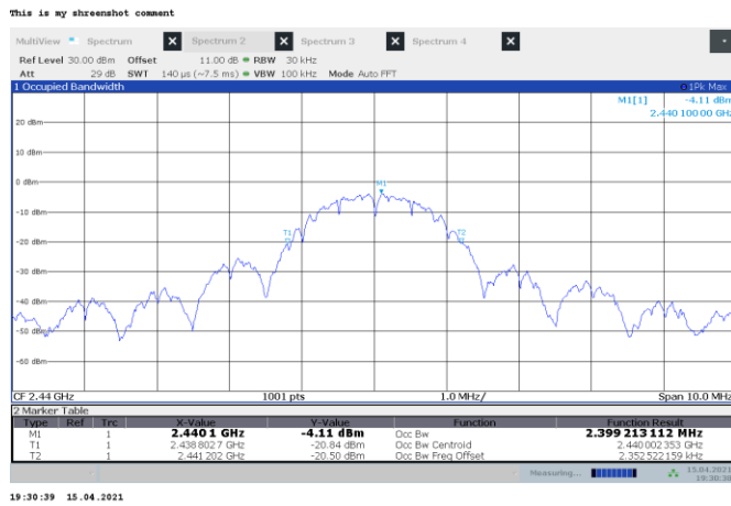
Figure 8.1-5: 99% occupied bandwidth on mid channel
