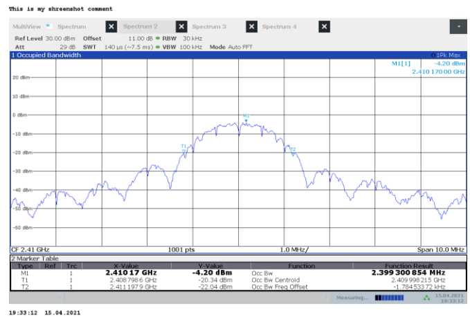
Figure 8.1-4: 99% occupied bandwidth on low channel
