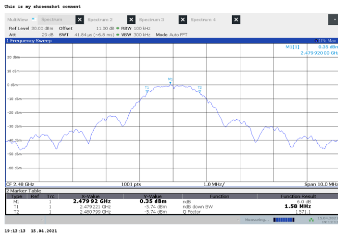
Figure 8.1-3: 6 dB bandwidth on top channel
