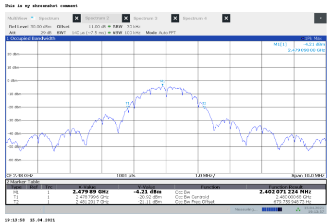
Figure 8.1-6: 99% occupied bandwidth on high channel
