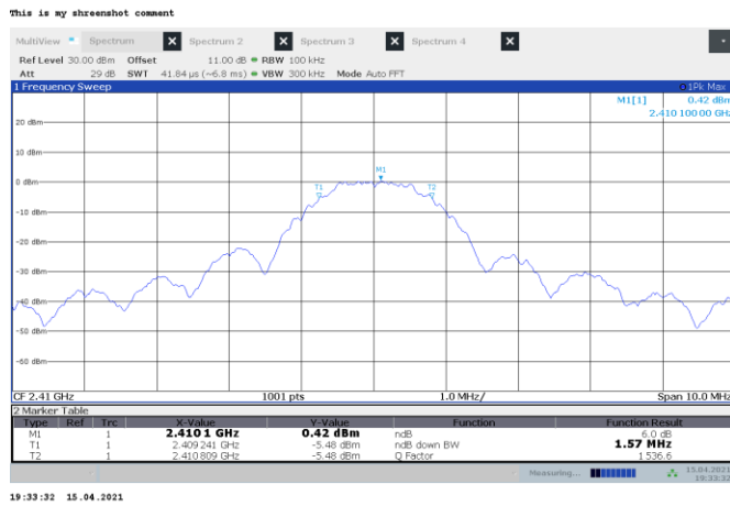
Figure 8.1-1: 6 dB bandwidth on low channel
