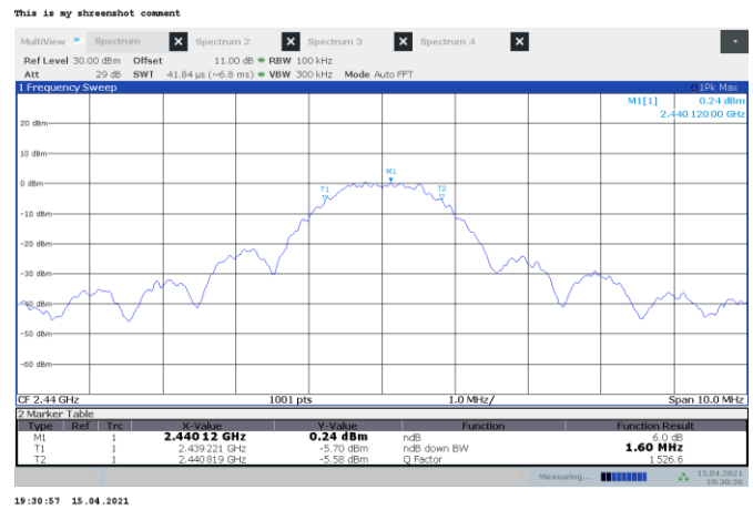
Figure 8.1-2: 6 dB bandwidth on mid channel
