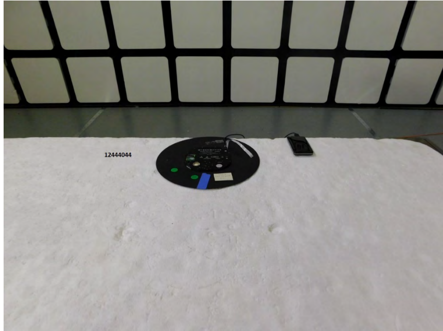
RADIATED SETUP PHOTO <1GHz TRANSMIT BATTERY
