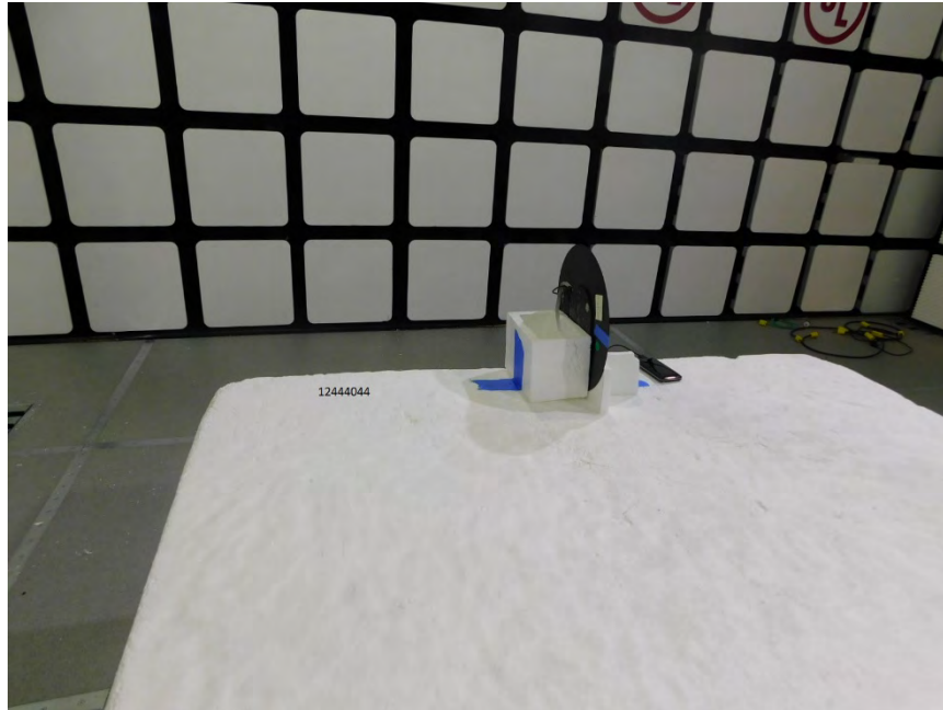
RADIATED SETUP PHOTO <1GHz RECEIVE BATTERY
