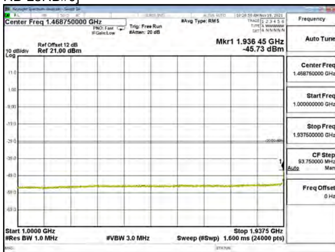
LTE BAND 01 - 5MHz - CH 1830 - QPSK[Full RB-25RB#0]
