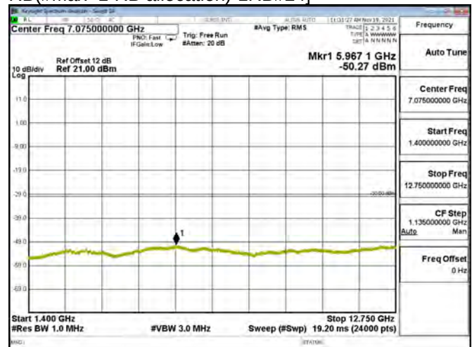
LTE BAND 08 - 5MHz - CH 21775 - QPSK[Partial RB(#Max+1-RB allocation)-1RB#24]
