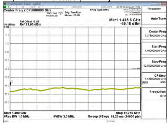
LTE BAND 28 - 5MHz - CH 27235 - QPSK[Partial RB(#Max+1-RB allocation)-1RB#24]
