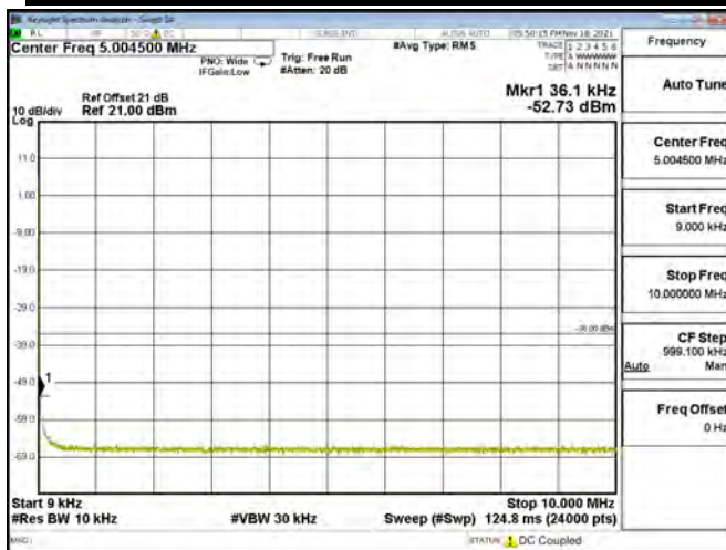
LTE BAND 07 - 20MHz - CH 21350 - QPSK[Full RB-100RB#0]
