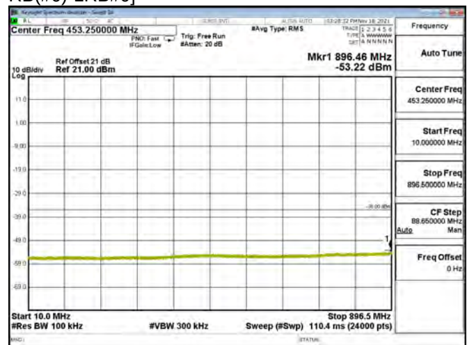
LTE BAND 08 - 1.4MHz - CH 21650 - QPSK[Partial RB(#Max+1-RB allocation)-1RB#5]
