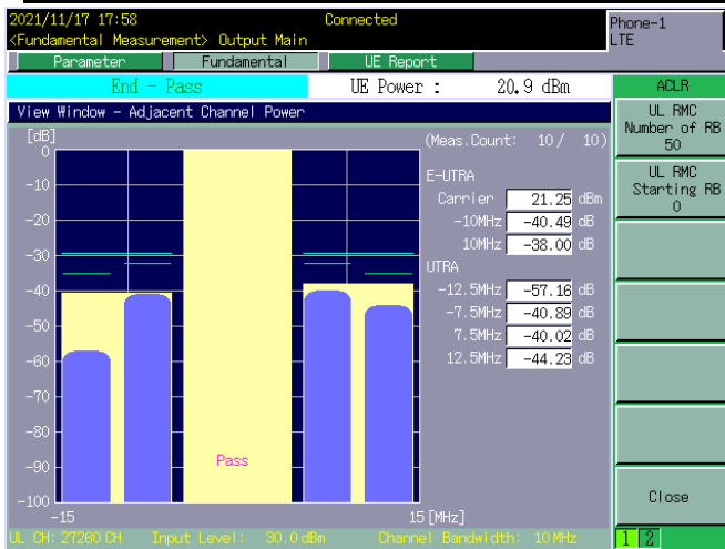
LTE BAND 28 - 10MHZ - CH 27260 - 16QAM[Full RB-50RB#0]
