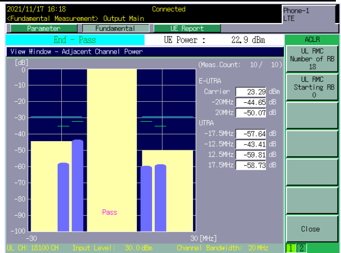
LTE BAND 01 - 20MHZ – CH 18100 - QPSK[Partial RB(#0)-18RB#0]
