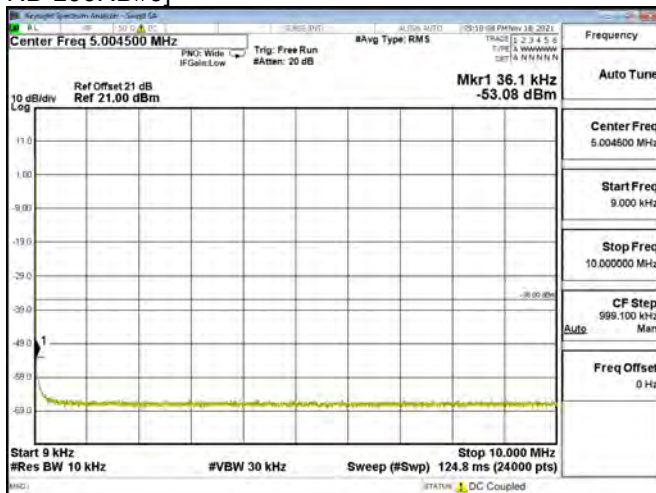
LTE BAND 01 - 20MHz - CH 18500 - QPSK[Partial RB(#0)-1RB#0]
