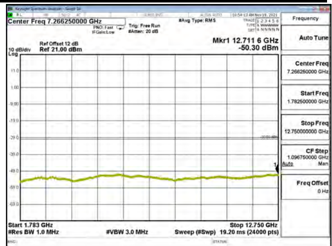
LTE BAND 03 - 20MHz - CH 19575 - QPSK[Partial RB(#0)-1RB#0]
