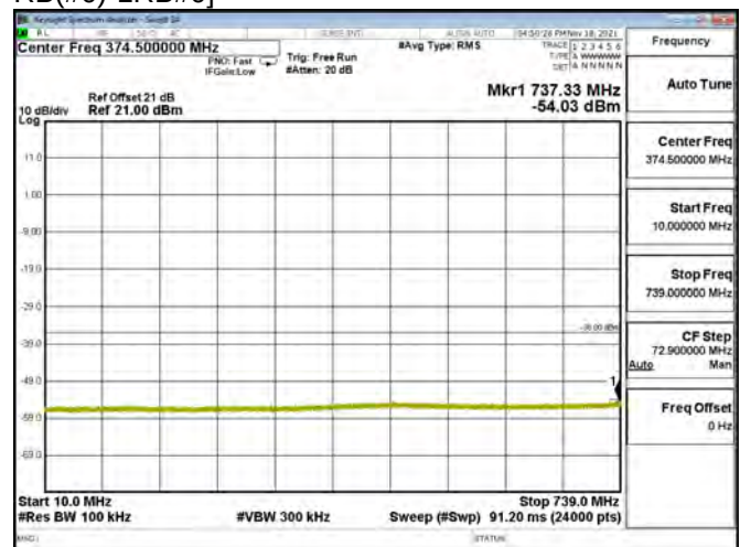
LTE BAND 28 - 3MHz - CH 27645 - QPSK[Partial RB(#Max+1-RB allocation)-1RB#14]
