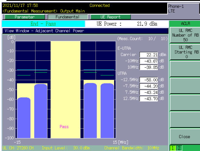
LTE BAND 28 - 10MHZ - CH 27260 - QPSK[Full RB-50RB#0]
