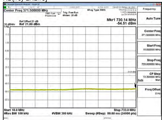
LTE BAND 28 - 5MHz - CH 27635 - QPSK[Partial RB(#Max+1-RB allocation)-1RB#24]
