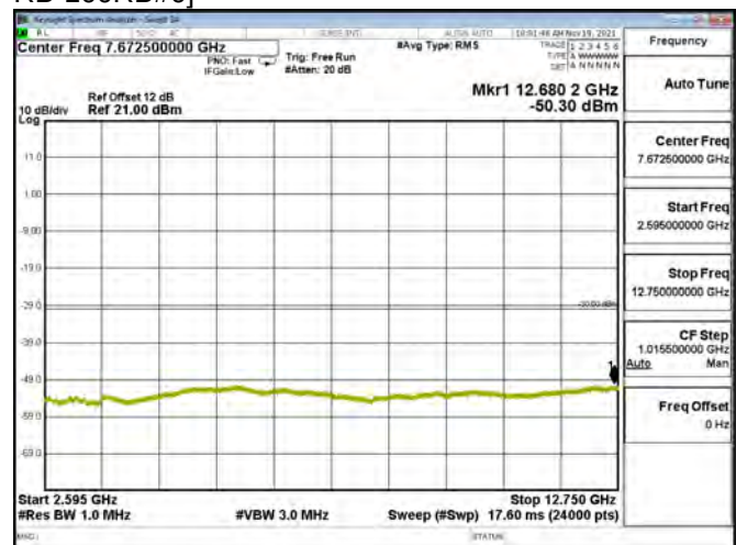
LTE BAND 07 - 20MHz - CH 21350 - QPSK[Full RB-100RB#0]
