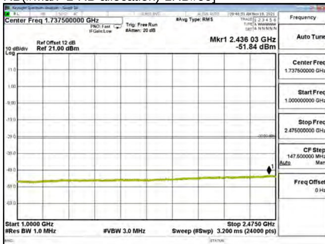
LTE BAND 07 - 20MHz - CH 20850 - QPSK[Partial RB(#Max+1-RB allocation)-1RB#99]
