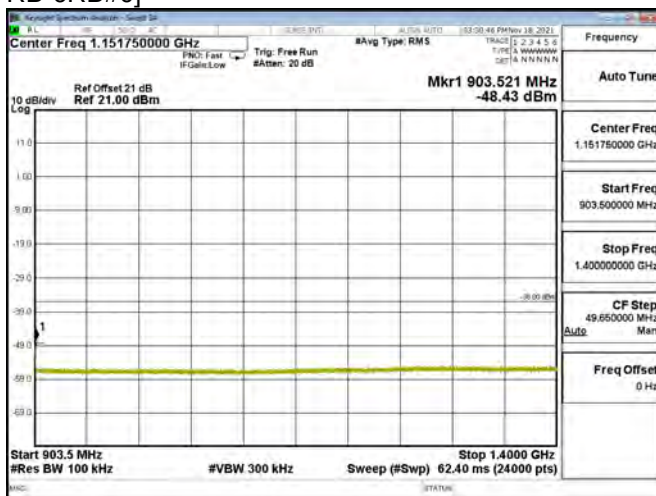
LTE BAND 08 - 1.4MHz - CH 21650 - QPSK[Full RB-6RB#0]
