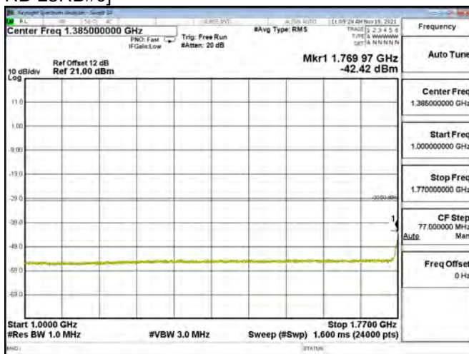
LTE BAND 03 - 5MHz - CH 19925 - QPSK[Full RB-25RB#0]
