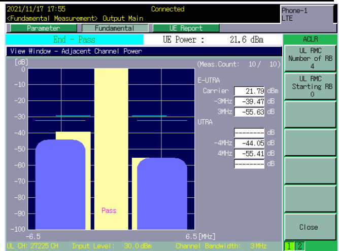
LTE BAND 28 - 3MHz - CH 27225 - 16QAM[Partial RB(#0)-4RB#0]
