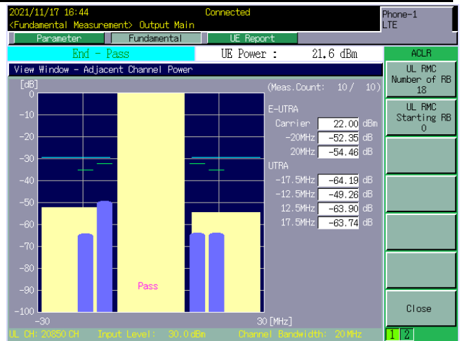
LTE BAND 07 - 20MHZ – CH 20850 - QPSK[Partial RB(#0)-18RB#0]
