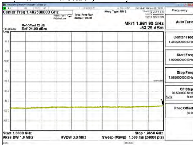
LTE BAND 01 - 5MHz - CH 18575 - QPSK[Partial RB(#Max+1-RB allocation)-1RB#24]
