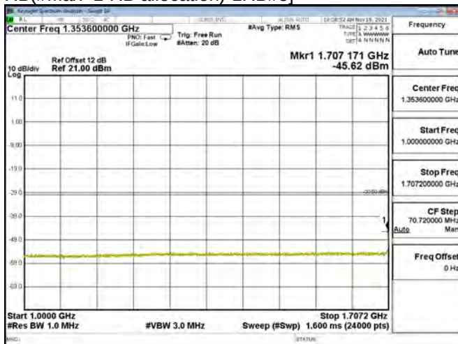
LTE BAND 03 - 1.4MHz - CH 19207 - QPSK[Partial RB(#Max+1-RB allocation)-1RB#5]
