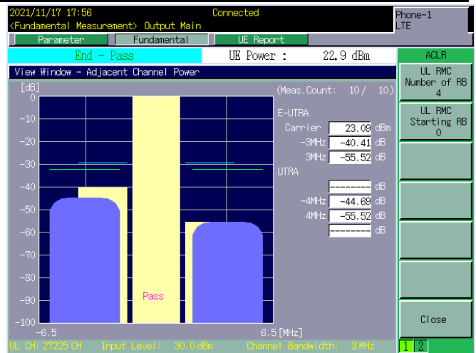
LTE BAND 28 - 3MHz - CH 27225 - QPSK[Partial RB(#0)-4RB#0]
