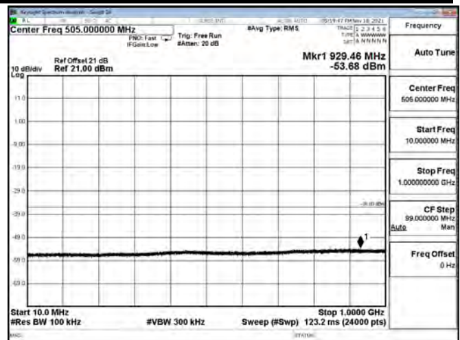
LTE BAND 03 - 5MHz - CH 19225 - QPSK[Full RB-25RB#0]
