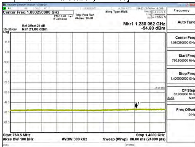
LTE BAND 28 - 20MHz - CH 27435 - QPSK[Partial RB(#Max+1-RB allocation)-1RB#99]
