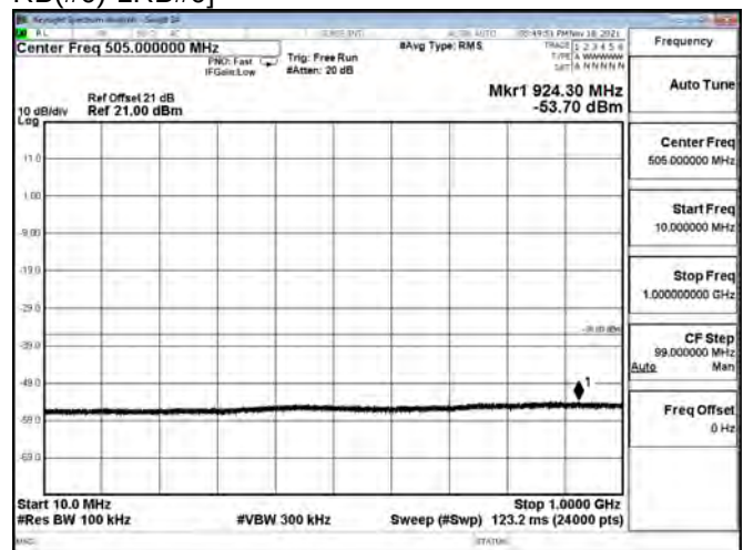
LTE BAND 07 - 20MHz - CH 21350 - QPSK[Partial RB(#Max+1-RB allocation)-1RB#99]
