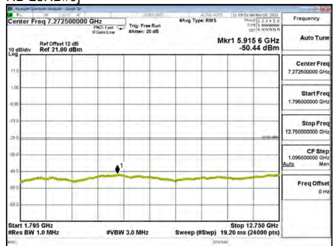
LTE BAND 03 - 5MHz - CH 19925 - QPSK[Full RB-25RB#0]
