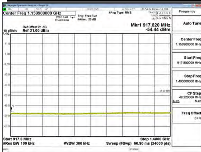
LTE BAND 08 - 1.4MHz - CH 21793 - QPSK[Partial RB(#0)-1RB#0]
