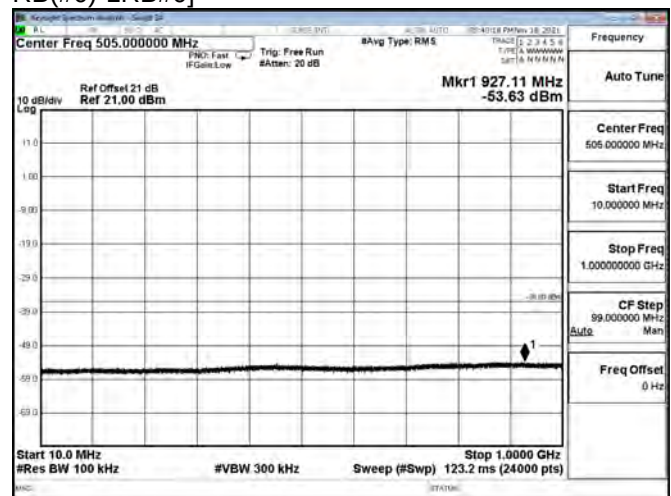
LTE BAND 07 - 5MHz - CH 20775 - QPSK[Partial RB(#Max+1-RB allocation)-1RB#24]
