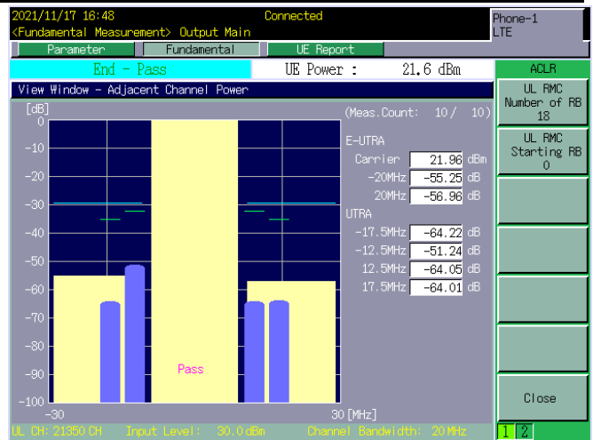
LTE BAND 07 - 20MHZ – CH 21350 - QPSK[Partial RB(#0)-18RB#0]
