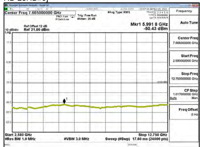
LTE BAND 07 - 5MHz - CH 21425 - QPSK[Full RB-25RB#0]
