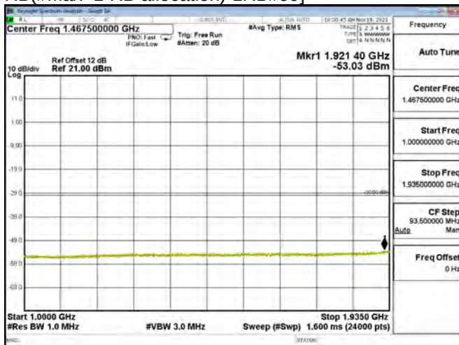
LTE BAND 01 - 20MHz - CH 18500 - QPSK[Partial RB(#Max+1-RB allocation)-1RB#99]
