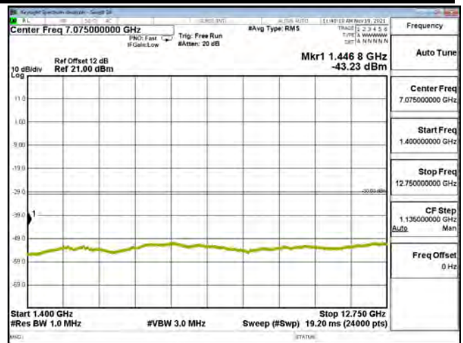
LTE BAND 28 - 5MHz - CH 27435 - QPSK[Partial RB(#0)-1RB#0]
