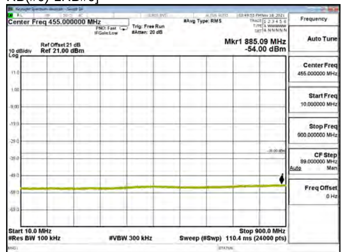
LTE BAND 08 - 5MHz - CH 21775 - QPSK[Partial RB(#Max+1-RB allocation)-1RB#24]
