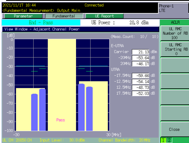
LTE BAND 07 - 20MHZ – CH 20850 - QPSK[Full RB-100RB#0]
