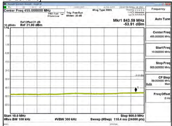
LTE BAND 08 - 5MHz - CH 21775 - QPSK[Partial RB(#0)-1RB#0]
