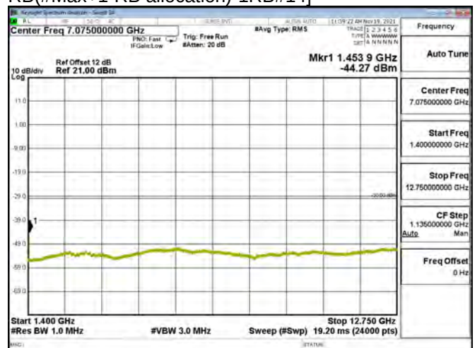
LTE BAND 28 - 3MHz - CH 27435 - QPSK[Partial RB(#Max+1-RB allocation)-1RB#14]
