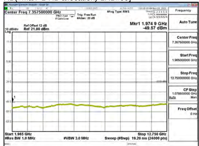
LTE BAND 01 - 20MHz - CH 18100 - QPSK[Partial RB(#Max+1-RB allocation)-1RB#99]
