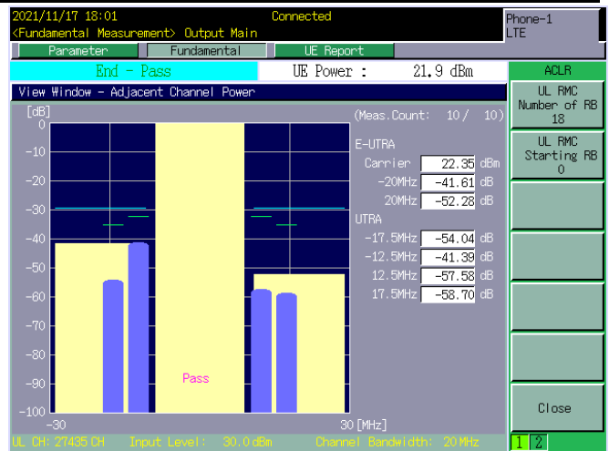
LTE BAND 28 - 20MHZ – CH 27435 - 16QAM[Partial RB(#0)-18RB#0]
