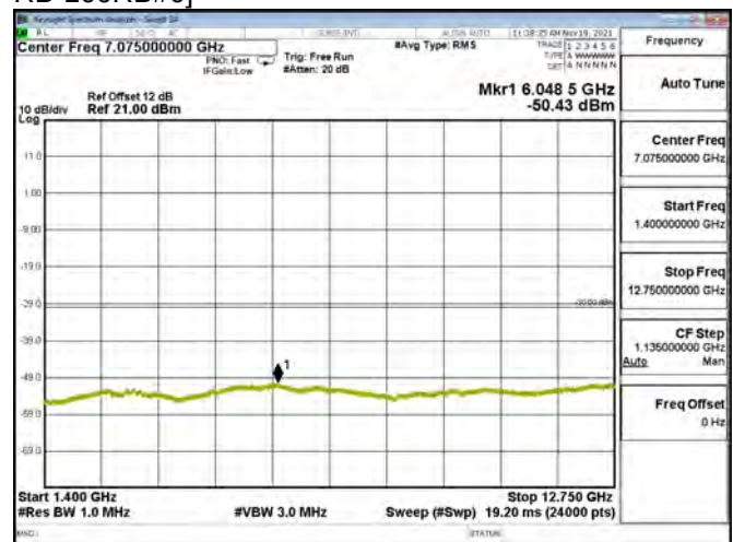
LTE BAND 28 - 20MHz - CH 27435 - QPSK[Full RB-100RB#0]
