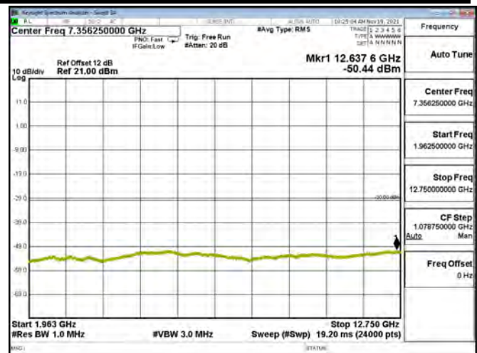
LTE BAND 01 - 5MHz - CH 1830 - QPSK[Partial RB(#0)-1RB#0]
