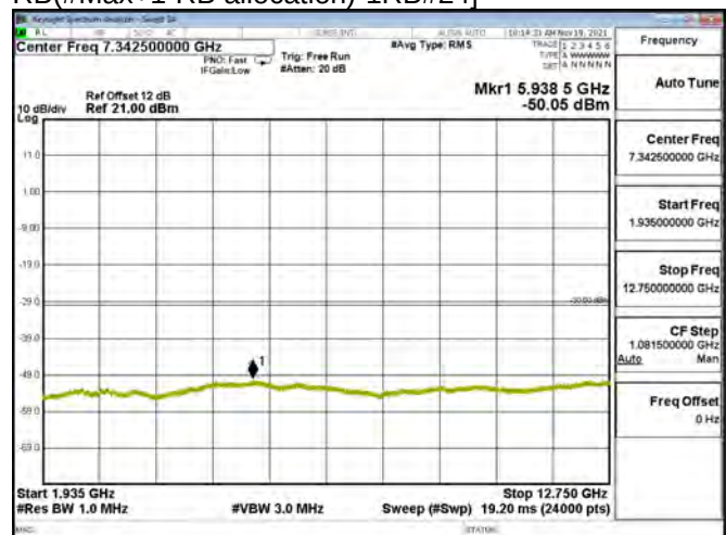
LTE BAND 01 - 5MHz - CH 18025 - QPSK[Partial RB(#Max+1-RB allocation)-1RB#24]
