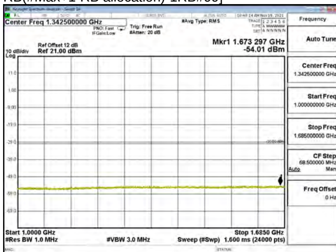
LTE BAND 03 - 20MHz - CH 19300 - QPSK[Partial RB(#Max+1-RB allocation)-1RB#99]
