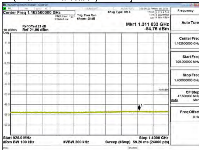
LTE BAND 08 - 5MHz - CH 21775 - QPSK[Partial RB(#Max+1-RB allocation)-1RB#24]
