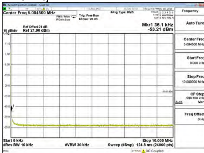
LTE BAND 03 - 5MHz - CH 19925 - QPSK[Partial RB(#0)-1RB#0]
