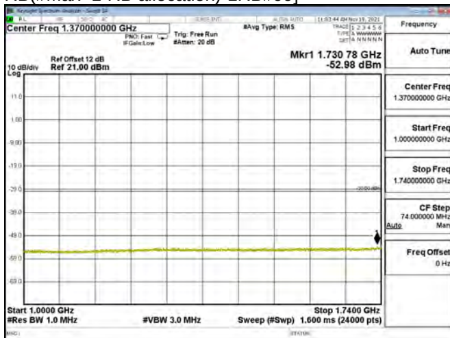
LTE BAND 03 - 20MHz - CH 19850 - QPSK[Partial RB(#Max+1-RB allocation)-1RB#99]
