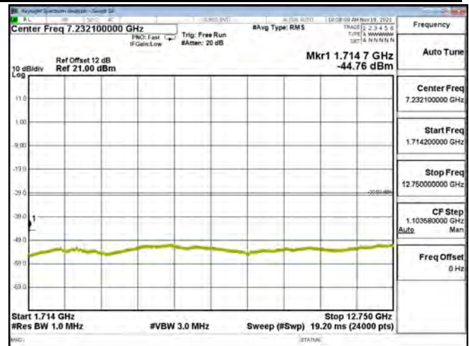
LTE BAND 03 - 1.4MHz - CH 19207 - QPSK[Partial RB(#0)-1RB#0]
