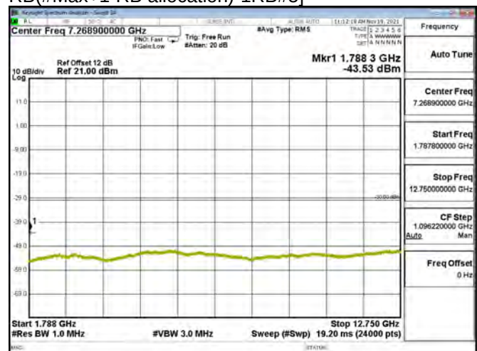
LTE BAND 03 - 1.4MHz - CH 19943 - QPSK[Partial RB(#Max+1-RB allocation)-1RB#5]
