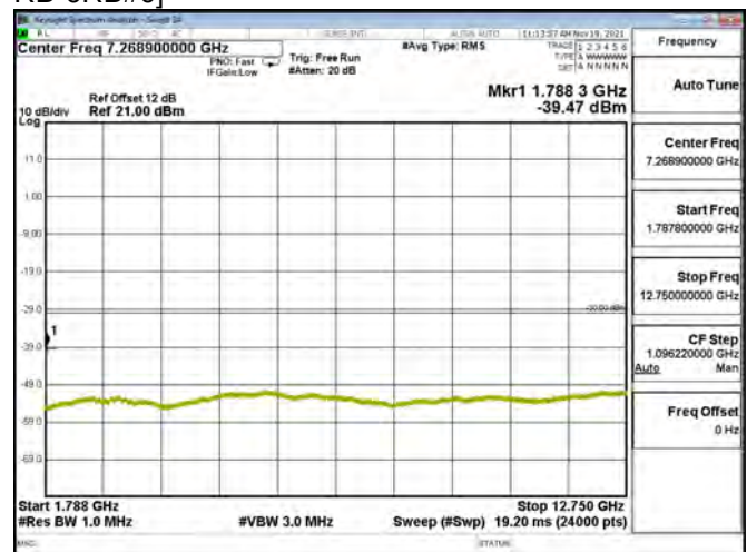
LTE BAND 03 - 1.4MHz - CH 19943 - QPSK[Full RB-6RB#0]
