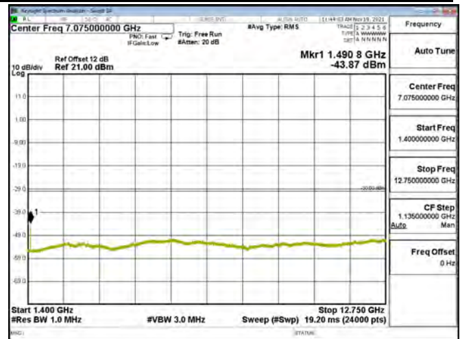
LTE BAND 28 - 3MHz - CH 27645 - QPSK[Partial RB(#0)-1RB#0]
