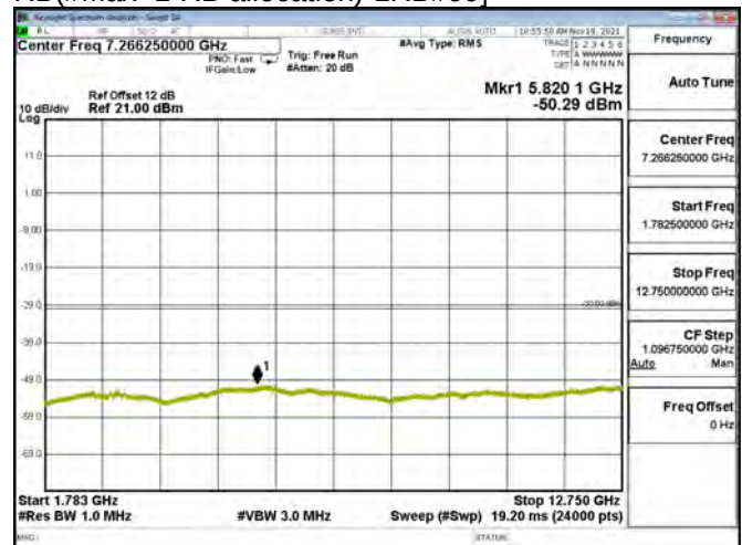
LTE BAND 03 - 20MHz - CH 19575 - QPSK[Partial RB(#Max+1-RB allocation)-1RB#99]
