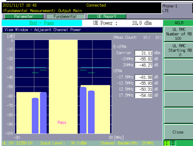
LTE BAND 07 - 20MHZ – CH 21350 - QPSK[Full RB-100RB#0]
