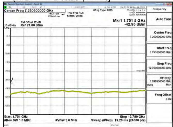
LTE BAND 03 - 1.4MHz - CH 19575 - QPSK[Partial RB(#Max+1-RB allocation)-1RB#5]
