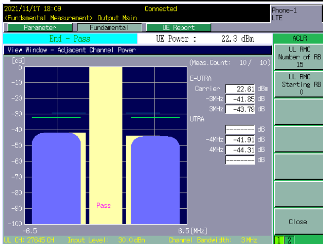
LTE BAND 28 - 3MHZ – CH 27645 - QPSK[Full RB-15RB#0]
