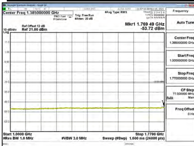
LTE BAND 03 - 5MHz - CH 19925 - QPSK[Partial RB(#0)-1RB#0]
