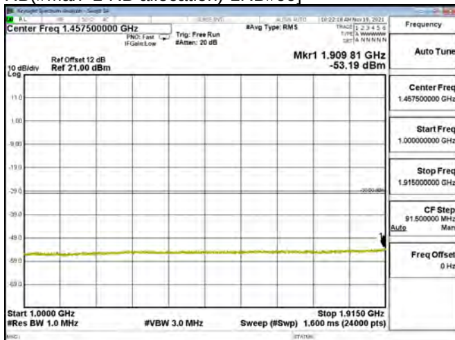
LTE BAND 01 - 20MHz - CH 18300 - QPSK[Partial RB(#Max+1-RB allocation)-1RB#99]
