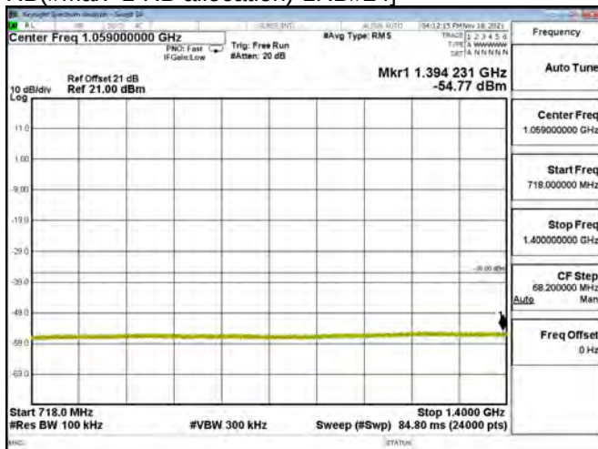
LTE BAND 28 - 5MHz - CH 27235 - QPSK[Partial RB(#Max+1-RB allocation)-1RB#24]
