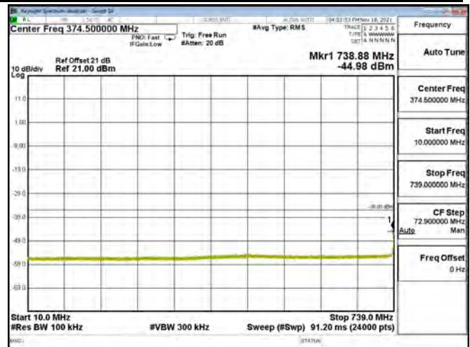
LTE BAND 28 - 3MHz - CH 27645 - QPSK[Full RB-15RB#0]
