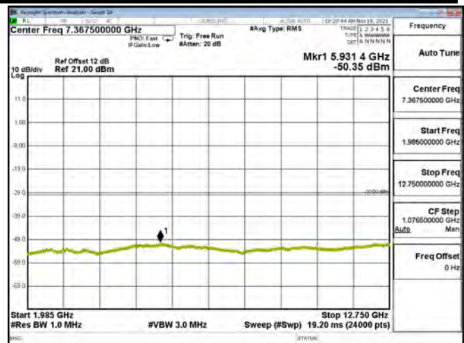
LTE BAND 01 - 20MHz - CH 18300 - QPSK[Partial RB(#0)-1RB#0]
